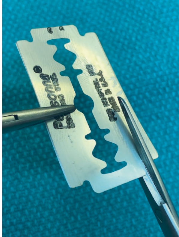
Fig. 5.10 Use heavy scissors to cut out the central arms of a safety razor blade, providing two long blades. (Photo Credit: Sheldon Marks)
