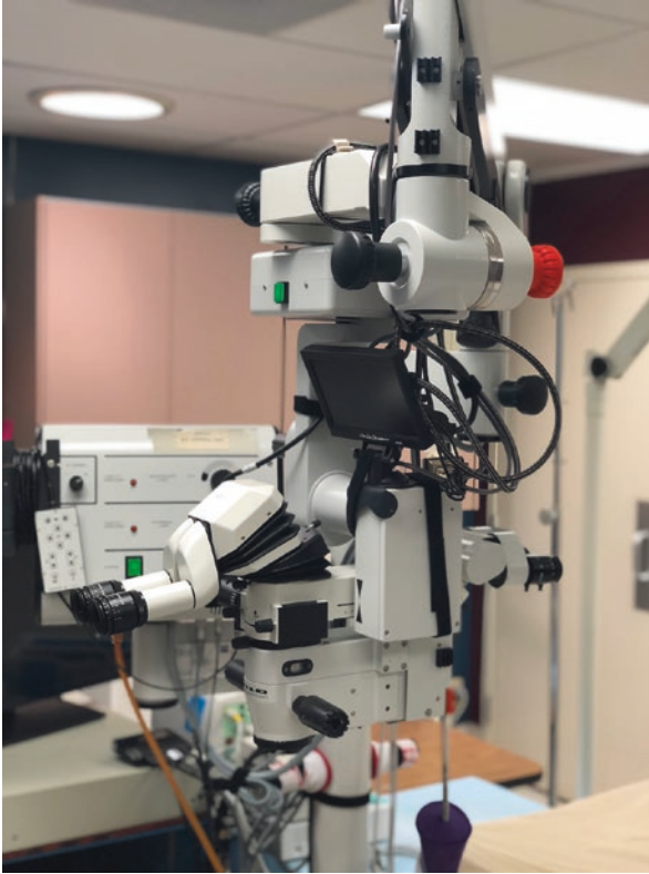
Fig. 3.1 Example of Leica XYdouble-headed, motorized focus and zoom foot-controlled surgical microscope. (Photo Credit: Sheldon Marks)
