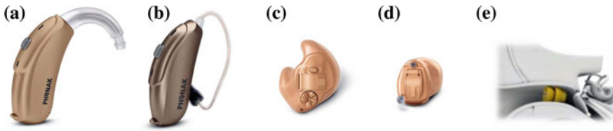
Fig. 1 Different types of state-of-the-art hearing aids. a BTE, b RIC, c ITE, d ITC, e CIC
