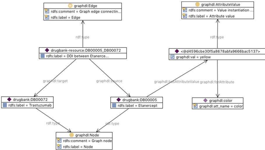
Fig. 1. Representation of vertices, edges and properties in GraphDL, example with DrugBank interaction Etanercept–Trastuzumab (created with TopBraid Composer TM )
