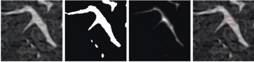
Fig. 5.8 Assessment of the trabecular thickness in a newly formed bone. From left to right: original image; segmented image; distance transform represented with gray level; overlaid maximal sphere. The local maximum of the distance transform can be considered the center of the maximal inscribed sphere, and this sphere can be also overlaid to the original image in order to visualize the point where the local thickness is assessed. For the sake of clarity, the concept is represented in 2D, but it applies to the 3D segmented domain
