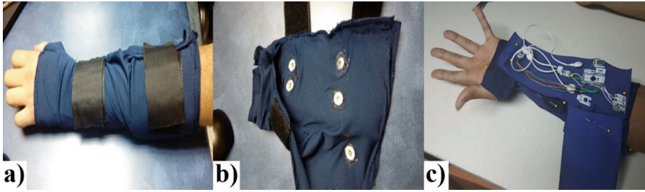
Fig. 1. Wearable sensor prototype. (a) View from outside. (b) EMG and EDA Electrodes. (c) Bitalino boards and electrodes inside the glove.
