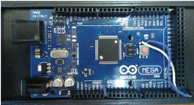
Fig. 3. Arduino MEGA employed in the present development.
