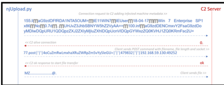
Fig. 6. Messages exchange for arbitrary file upload to C2 server.
