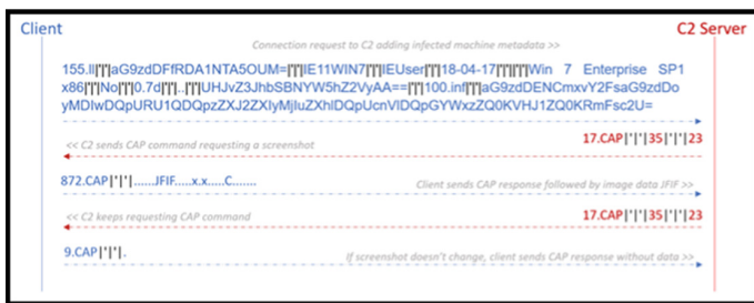
Fig. 3. Communication establishment between bot and C2 server.
