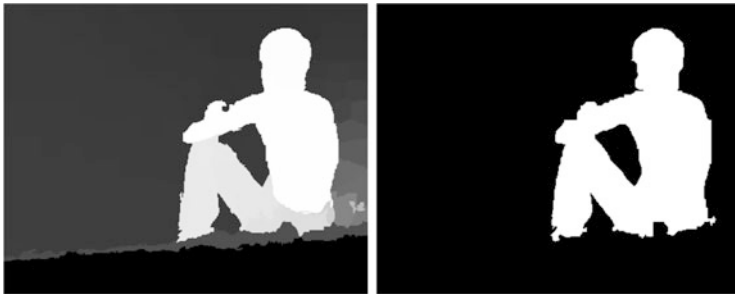
Fig. 7 Saliency cut algorithm in an image from MSRA10K benchmark. On the left hand side our NLTV + SCALP + Bon and right hand side the result of applying SaliencyCut to this saliency map
