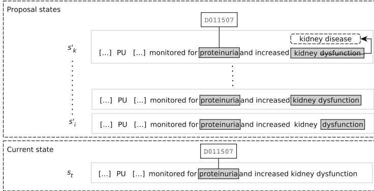
Fig. 7. Subset of proposal states generated by the segmentation explorer, originating from the current state s_t which has already one linked segmentation on token t_{13} . Each proposal state has a new non-overlapping segment annotation (marked in grey) that is not linked to any concept. Proposal states may include synonym replacements (depicted as dashed boxes) that are accepted for all subsequent sampling steps.
