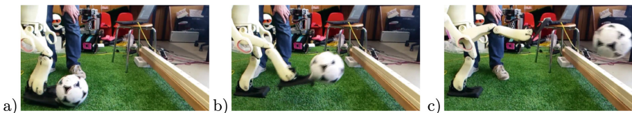
Fig. 13. Robot performing a high kick over a 21 cm obstacle. (a) The ball is being scooped by the foot. (b) The ball is kicked upwards. (c) The ball overcame the obstacle.
