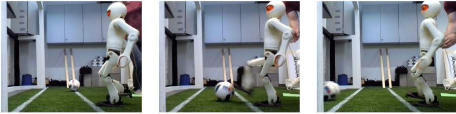
Fig. 14. Robot scoring from a moving ball. Left: the robot is waiting for the ball. Middle: the kick is executed. Right: a goal is scored.
