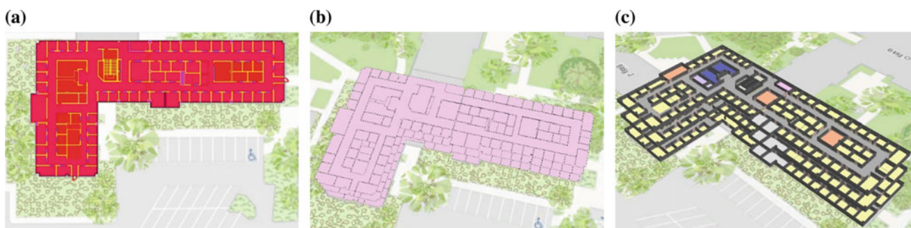
Fig. 75.2 a 2D building floorplan, b 3D building floorplans, c 3D building form with space classification as polygons (The Authors, 2018)
