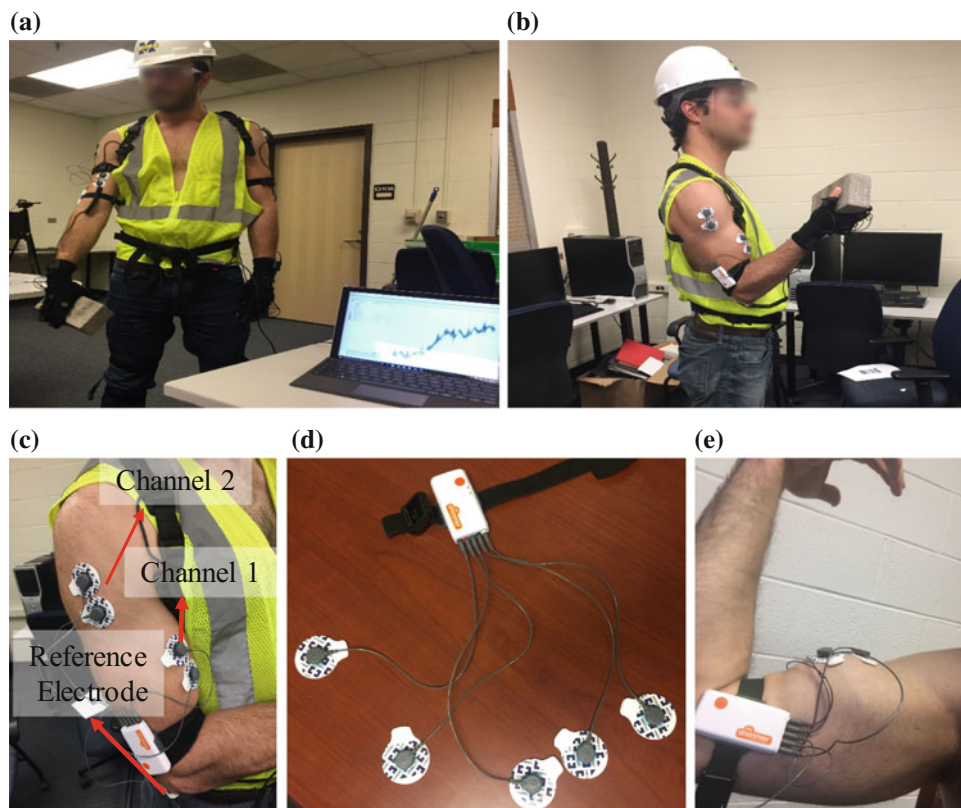
Fig. 22.2 Experimental setup: a Task 1: lifting concert brick using shoulder muscle; b Task 2: lifting concrete block using bicep muscle; c Placement of EMG channels; d An off-the-shelf wearable EMG sensor that was used in this study; e Placement of EMG electrodes on muscle peak
