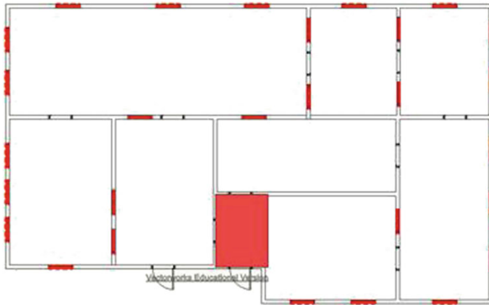
Fig. 11.4 The highlighted room violates the minimum area rule
