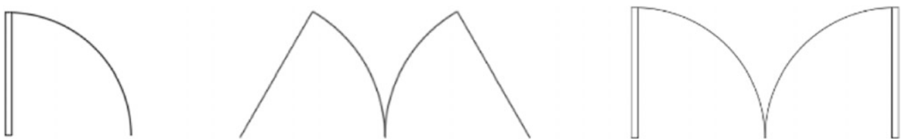
Fig. 9.5 Different shapes of door in real-life 2D drawings
