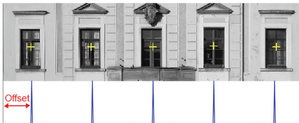
Fig. 64.3 Dirac comb (blue) shifted by an offset (red) to match the windows' centers (yellow crosses)
