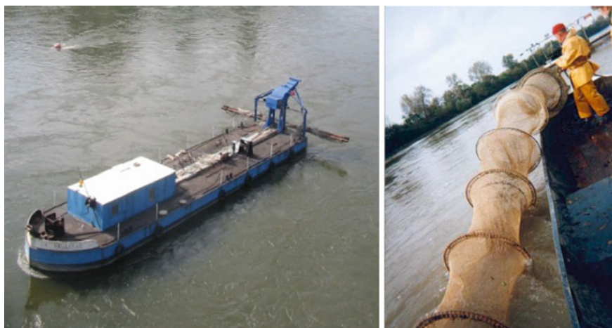
Fig. 7.15 Fishing gear used to catch the silver eel in the Loire River. It is an anchored stownet called “Guideau” (E. Feunteun)
