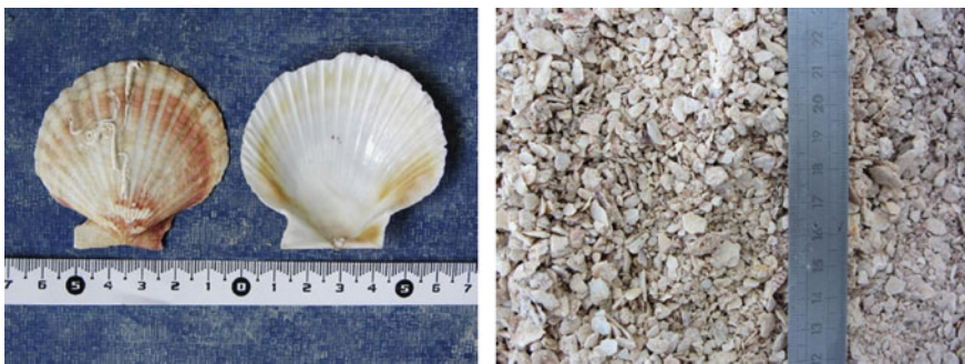
Fig. 22.1 Queen scallop Aequipecten opercularis (Linnaeus 1758) and crushed queen scallop shells used to make up the substrate of concrete blocks (after Cuadrado et al. 2015)
