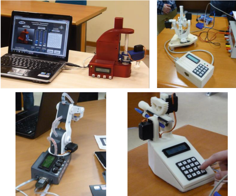
Fig. 2. Manipulators built by the students.
