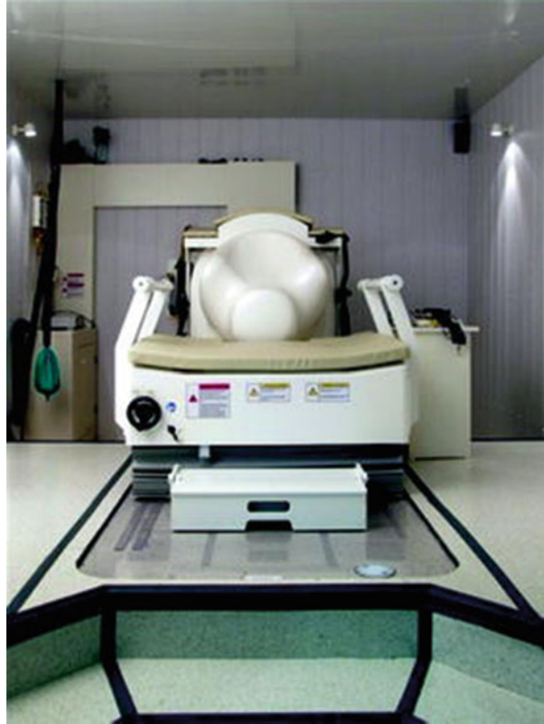
Fig. 1 156-channel fMEG device SARA II (SQUID Array for Reproductive Assessment, VSM MedTech Ltd., Port Coquitlam, Canada) installed at the fMEG Center in Tübingen. (© University Hospital Tübingen)
