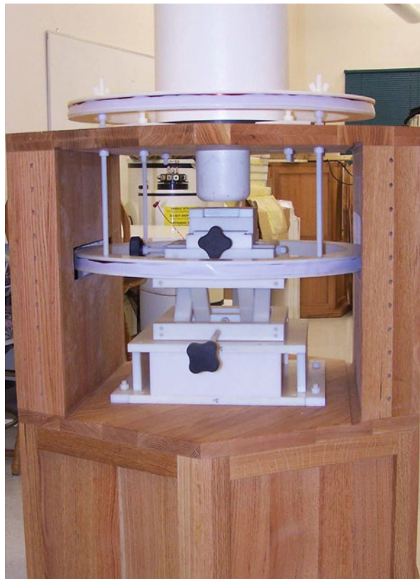
Fig. 1 Photograph of magnetic relaxometry system used at Senior Scientific for studying disease using cell cultures and small animals. The upper structure is the dewar containing the SQUID sensors with gradiometers in the protruding snout. The Helmholtz coils are shown above and below the measurement stage
