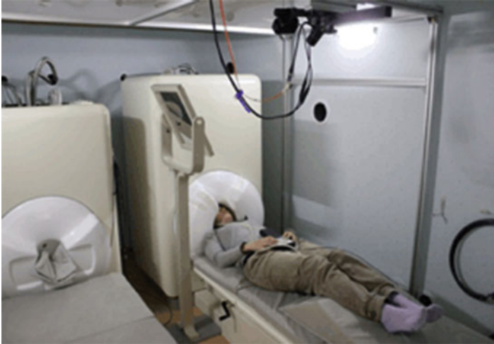
Fig. 2 Separate child (left) and adult (right) MEG systems contained within a single large MSR. A novel alternative configuration has child and adult helmet dewars at opposite ends of a single, swiveling, helium dewar ( https://compumedicsneuroscan.com/update-new-video-uploaded-orion-lifespan-meg/ ) which can be accommodated within a standard-sized MSR
