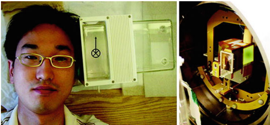
Fig. 28 A wide cell atomic brain magnetometer system for the purpose of source localization
