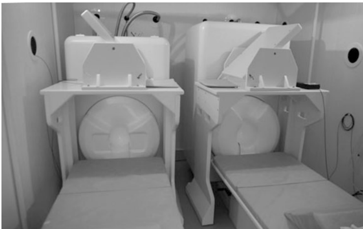
Fig. 2 Photograph depicting the child MEG system (left) and the conventional MEG system (right)
