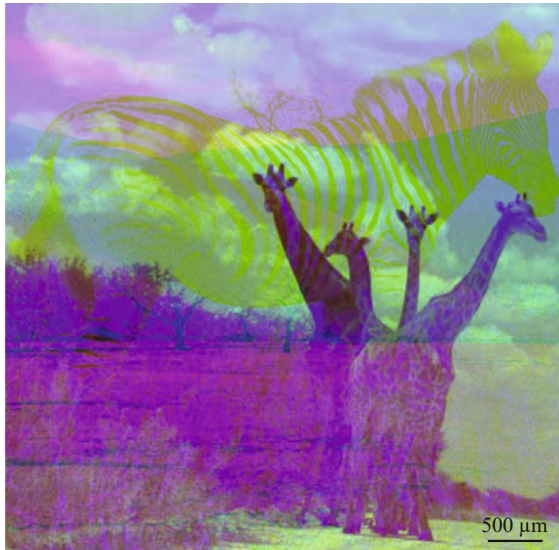
Fig. 17.58 The test specimen used in Fig. 17.57, an old-fashioned projector slide consisting of three superposed images, each of a different color. The dyes do not absorb perfectly at the laser frequencies in Fig. 17.57, so there is cross-talk in the reconstructions in Fig. 17.60. Reprinted from [17.54], with permission from Elsevier
