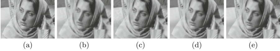
Fig. 2. Recovered Barbara with 5% sampling rate. (a) Original image; (b) NLR recovery (29.79 dB); (c) WNN recovery (30.54 dB); (d) TSPN recovery (30.63 dB); (e) TWSP recovery (30.81 dB).
