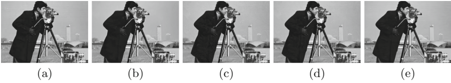
Fig. 5. Recovered Cameraman with SNR = 35 dB. (a) Original image; (b) NLR recovery (35.77 dB); (c) WNN recovery (37.04 dB); (d) TSPN recovery (36.99 dB); (e) TWSP recovery (38.11 dB).
