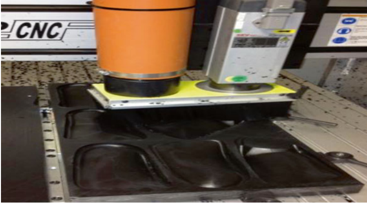
Fig. 21.3 Manufacturing four pairs of foot orthoses (homopolymer polypropylene for CAD-CAM)
