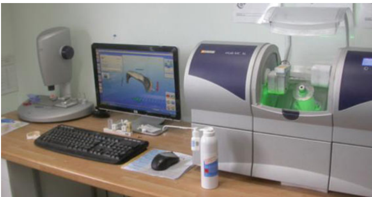
Fig. 15.16 Indirect Prosthodontic optic Process. From left to right : scan, C.A.D. unit, milling unit
