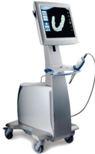
Fig. 15.15 The Lava C.O.S®. Intraoral Imprint unit for semi-direct C.A.D. – C.A.M.
