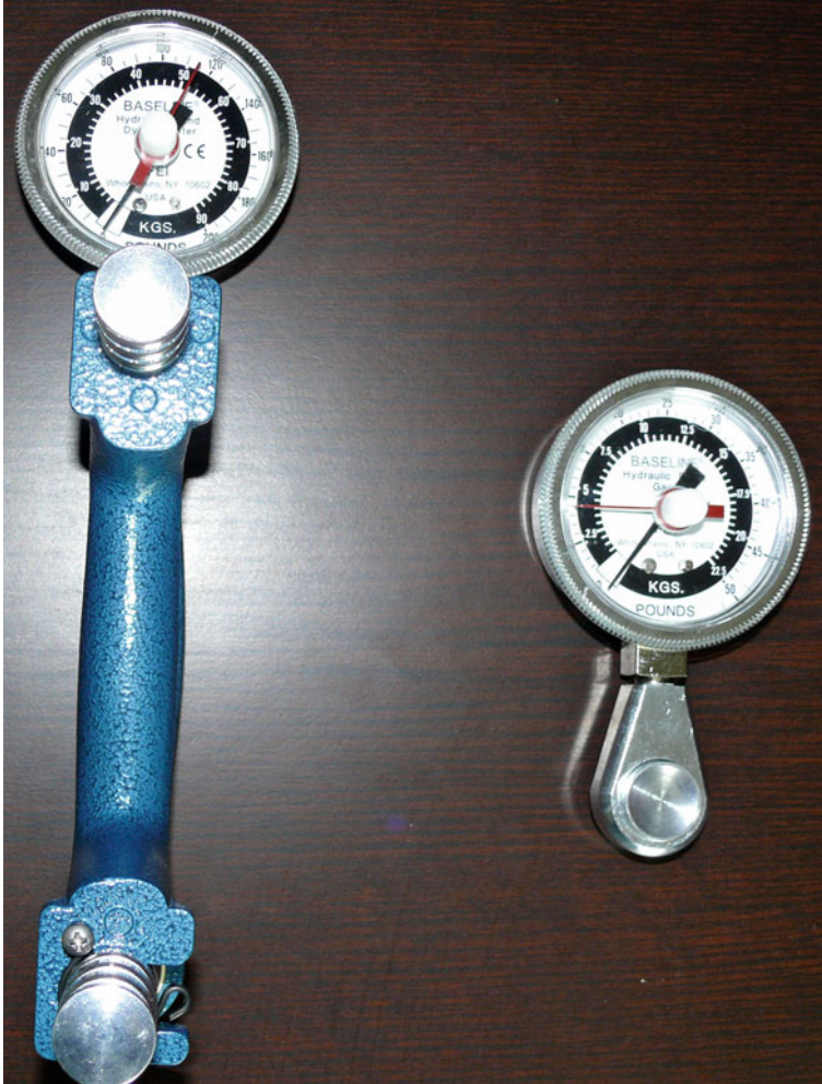
Fig. 7 Jamar dynamometer for grip strength measurement and pinch gauge dynamometer for pinch grip measurement
