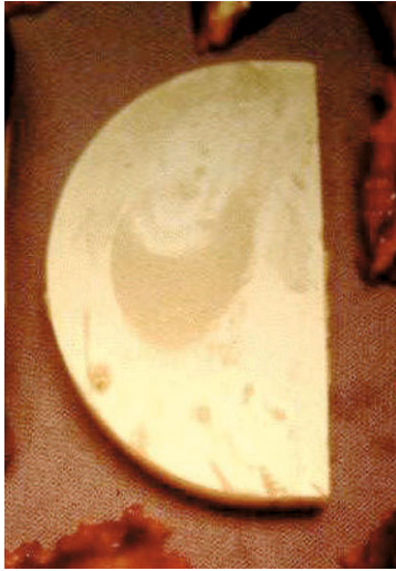
Fig. 1 – Retrieved flat tibial component (infected knee) demonstrating an early superficial wear track.
