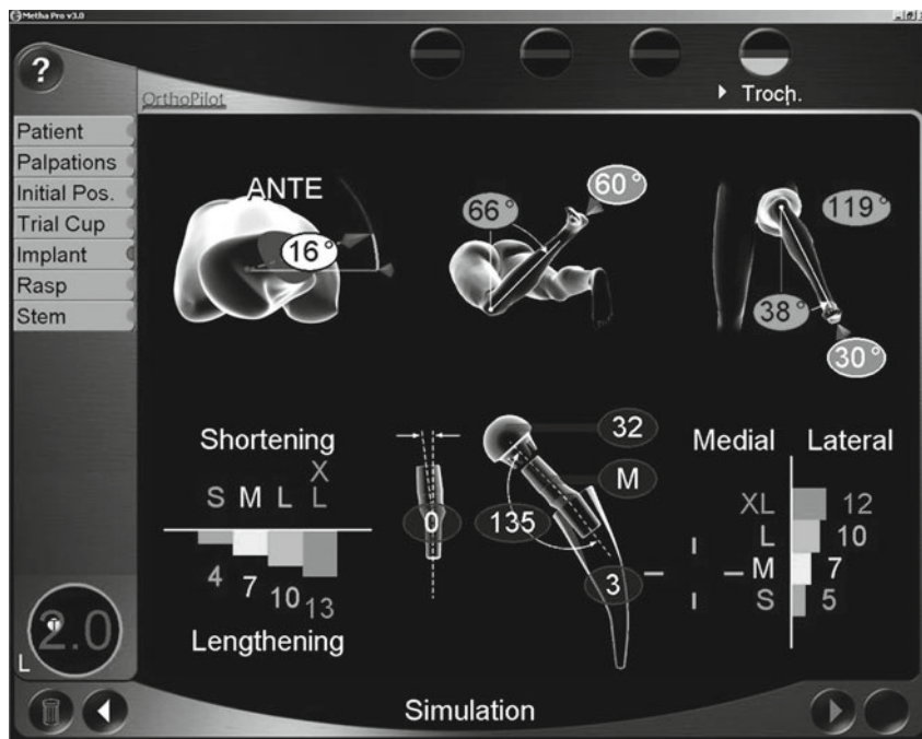
Fig. 13.10 The simulation screen of the navigation gives information on the mechanical changes influenced by the choice of the modular neck. In the centre, the antetorsion (here 0^\circ ) and the CCD angle (here: 135^\circ ) can be varied. The effect can be seen on the three pictures above: the antetorsion, the safe ROM for external rotation of the extended leg, and the safe ROM for internal rotation for the hip flexed at 90^\circ . It is also influenced by the head size. The offset and leg lengthening changes are displayed for all different head neck lengths
