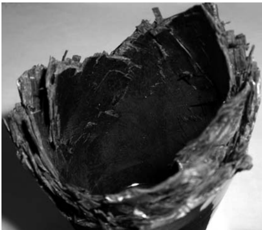
Figure 1 - Complete separation of handle and barrel for Bat ID C2.
