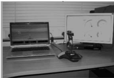
Figure 1 - Basic Display Environment, BDE showing instruments on laptop and VR on standard monitor.
