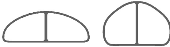
Figure 4 - Typical sections at the point of load for span A (left) and B (right).
