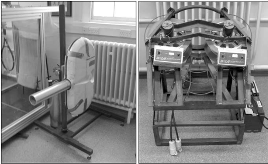
Figure 3 - The tennis BOLA machine and the football BOLA machine.
