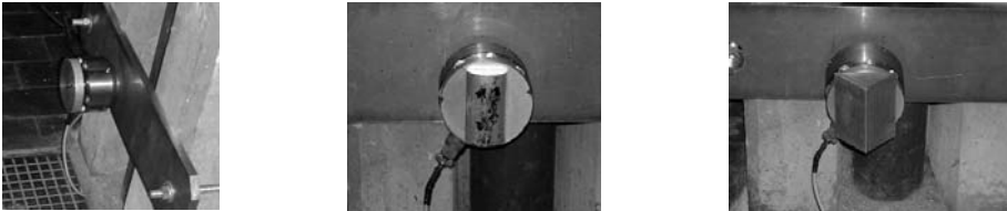
Figure 3 - Types of obstacle: Flat, Round (20mm radius) and Prismatic (90° edge angle; 1 mm fillet radius).
