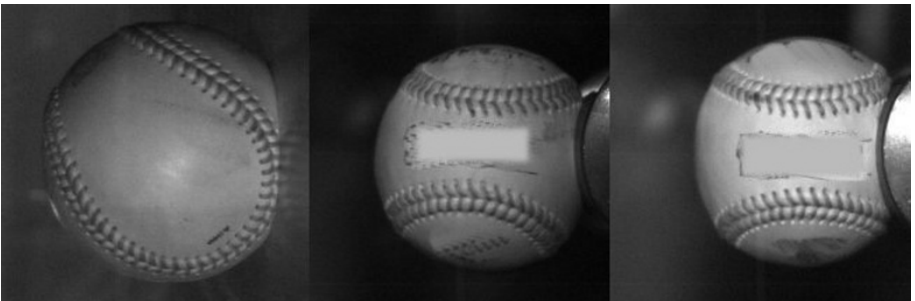
Figure 5 - High-speed video frames of impact for Model C [Left: 26.8 m/s (60-mph) COR, Middle: 26.8 m/s (60-mph) CCOR, and Right: 40.2 m/s (90-mph) CCOR].
