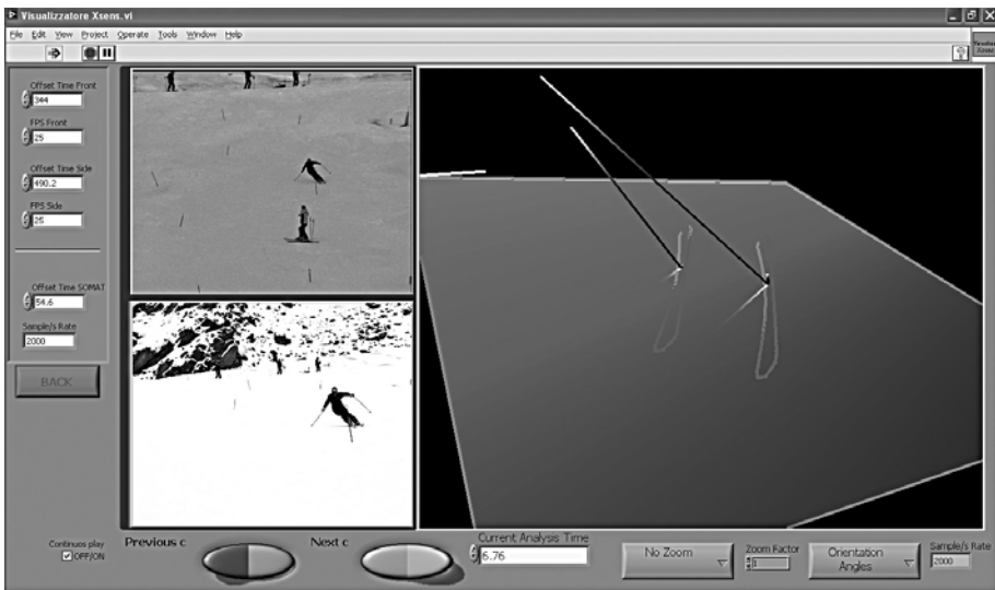
Figure 9 - Integrated analysis software application showing the instantaneous deformed shape of the ski and its instantaneous orientation with respect to the snow surface.
