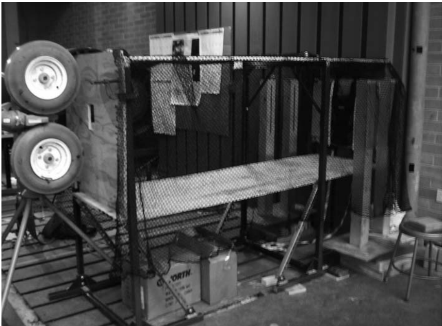
Figure 2 - Pitching machine COR setup.
