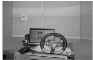
Figure 2 - Advanced Display Environment, ADE, showing wheel and curved display panels for VR driven by three data projectors.
