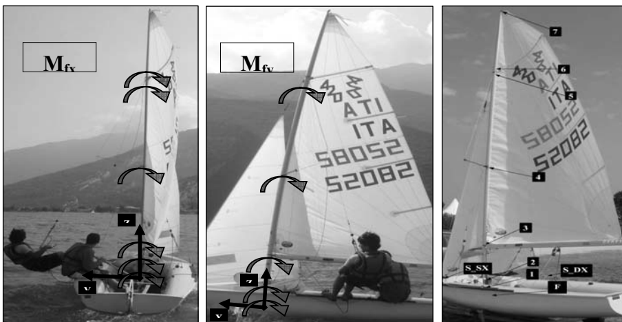
Figure 3 - (a) Lateral plane and M_{fx} measured. (b) Longitudinal plane and M_{fy} measured. (c) Global view of measuring points. Axial load F_z , not represented in the above pictures, was measured at mast sections 1, 2, 3, 5, 6, 7 and at mast step F.
