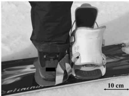
Figure 2 - Free foot standing on the anti-slip pad with rim next to the binding. The front of the board is on the left side.
