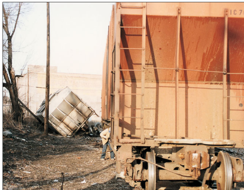
Fig. 4.10. A grain train wrecked due to a rail broken by severe cold conditions.
