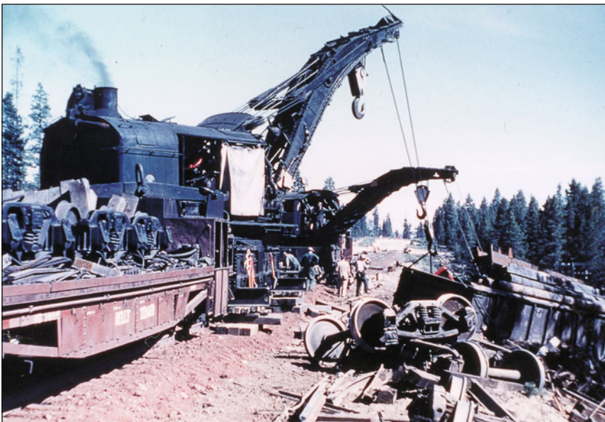
Fig. 5.15. Twin wreckers of the NP are lifting lumber cars derailed by a flood-caused washout in Idaho.
