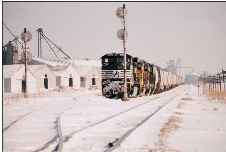
Fig. 2.10. Snow, high winds, and cold collectively are a major problem for railroads. Here a westbound NS train that had entered an Indiana siding to meet with an eastbound train has become stalled by drifts and cold temperatures on a morning with temperatures of -2^{\circ}\text{F} and winds of 35 mph.
