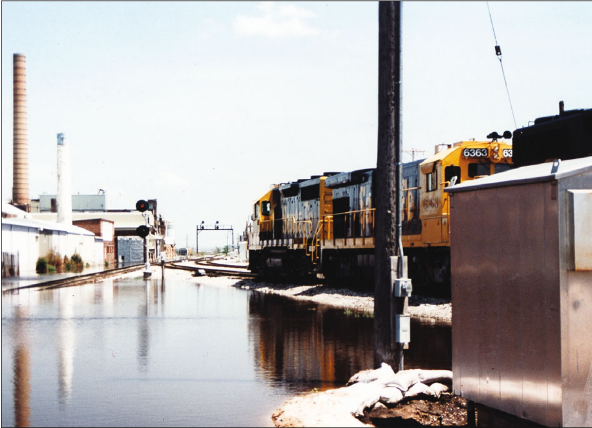
Fig. 2.9. The massive floods of the summer of 1993 in the Midwest caused huge damages. Here we see the Santa Fe's yards at Ft. Madison, Iowa, about to go under water as a train passes slowly on 2 July. Three days later the line here was closed. Note the sandbags around the control shed.
