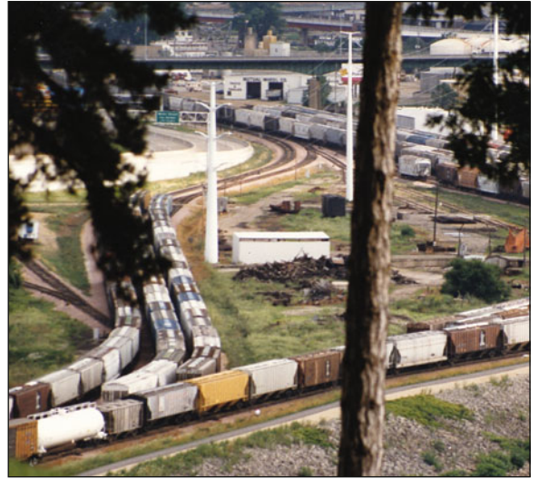
Figs. 2.2a and 2.2b. After the many locals service on-line elevators to get grain, the loaded cars are assembled in yards to either form grain trains to go to southern port cities or to deliver cars to riverside barge-loading facilities. In Fig. 2.2a (left), two SD40-2s of the Soo line at the Dubuque, Iowa yards are assembling a grain train for movement south. The Soo served many hundreds of grain elevators in the upper Midwest. Fig. 2.2b (right) shows an elevated view of the Dubuque yards, which are filled with loaded grain cars in October.
