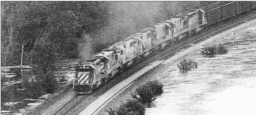
Fig. 3.7. A BN coal train, diverted north to Minneapolis because of a bridge closure at Burlington, Iowa, crawls alongside the flooded Mississippi River on 12 July 1993. Note the light-colored rock alongside the track close to the encroaching river, new gravel brought to protect the track from the flood.
