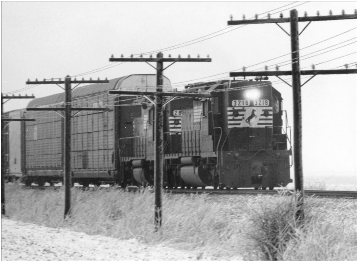
Fig. 2.15. Freezing rain brings several problems to railroads, including slippery rails and loss of traction. Here an NS train behind an SD40 and a GP38 heads slowly across southern Indiana after an ice storm ended. Note the ice on the wires, poles, and weeds.
