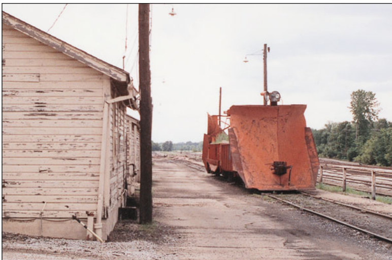
Fig. 5.8. Snowplows take on several configurations. The simplest form is seen here—a simple wedge mounted on a hopper car that gets pushed by an engine when in use. Note the light atop the plow for night operations.
