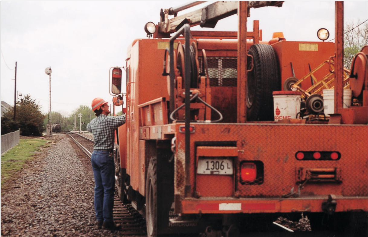
Fig. 5.2. Frequent observations of rails, ties, and roadbed are performed by track inspectors who move along rail lines in trucks such as this one in Minnesota.
