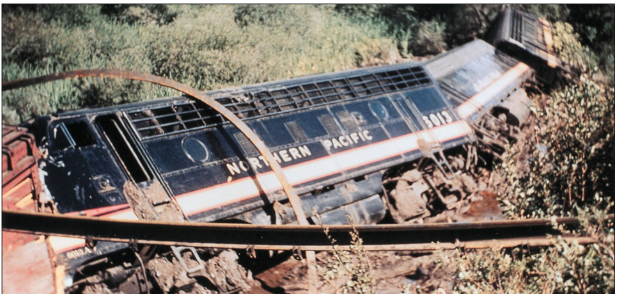
Fig. 4.17. A flash flood on a mountain stream in Montana washed out mainline tracks, resulting in the badly bent rails on the NP, causing the three locomotives leading a freight train west to derail and fall down this embankment.
