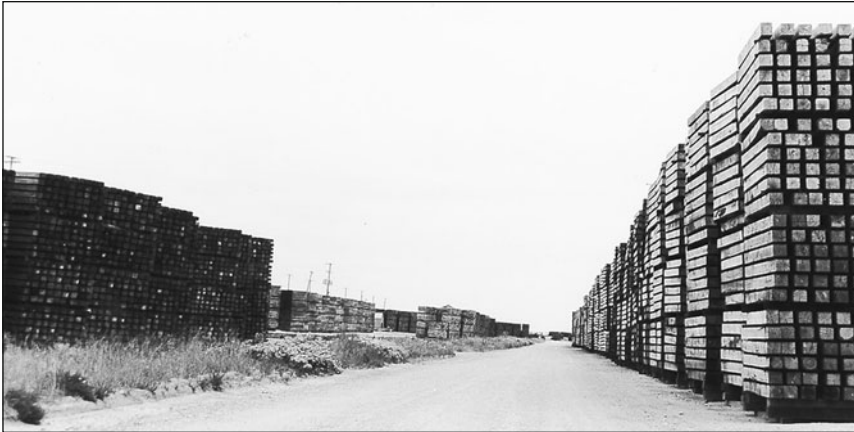
Fig. 5.13. All ties are weather-proofed. The process begins with several months of storage to let the moisture in the wood dry out. Then the ties are treated by creosote inserted under pressure.
