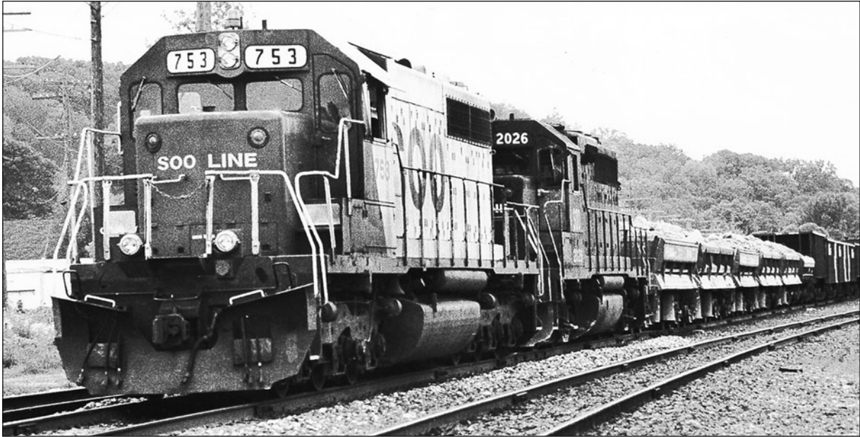
Fig. 5.16. A special Soo work train with cars loaded with rock excavated from the river bluffs near Savanna, Illinois, heads along the Mississippi River shore on 13 July 1993. The rock was dumped along the railroad's vulnerable river line near Davenport, Iowa.
