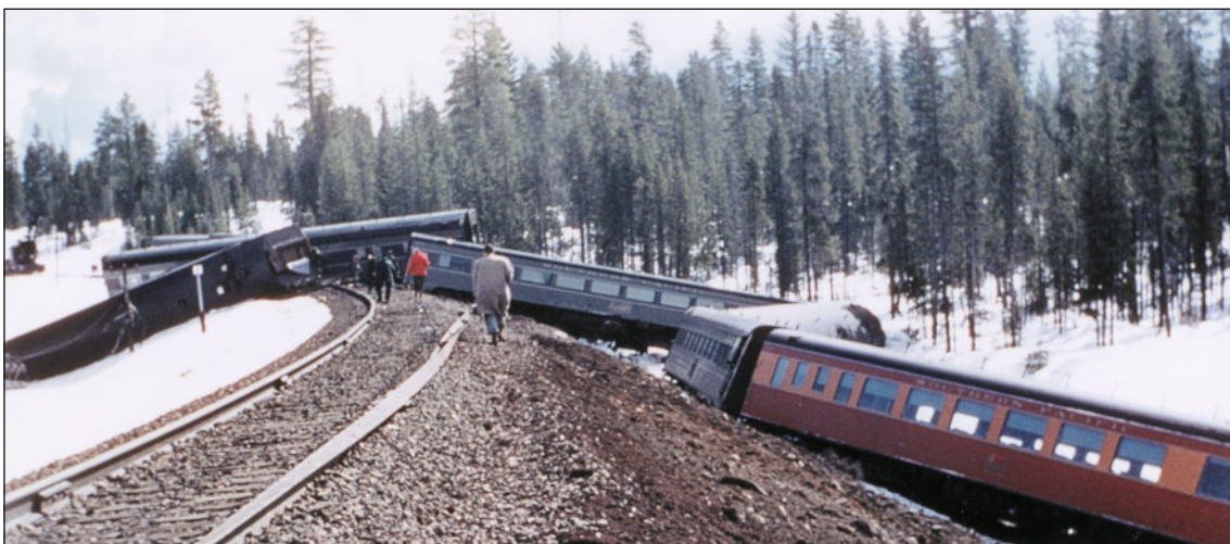
Fig. 4.12. A broken rail from the severe cold on the Shasta Line of the SP in the mountains of northern California caused this major wreck of the "Cascade."
