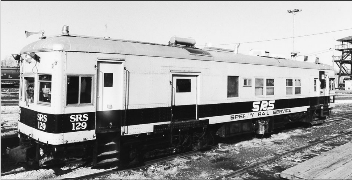
Fig. 5.1. One of the many weather-related preventive actions railroads take is to check roadbeds using sensors in special cars operated by the Sperry Rail Service. Here, one such car is parked on a North Carolina siding awaiting permission to begin measurements along an NS line.
