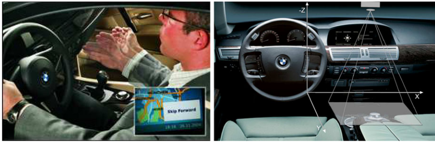
Fig. 14 BMW’s gesture control prototype [11]. (Left) skipping audio tracks by hand gestures; (Right) reference coordinate system for hand gestures with interaction area
