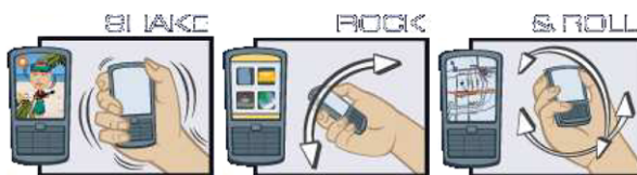
Fig. 13 The EyeMobile engine from GestureTek [86] tracks three movements: shake, rock, and roll
