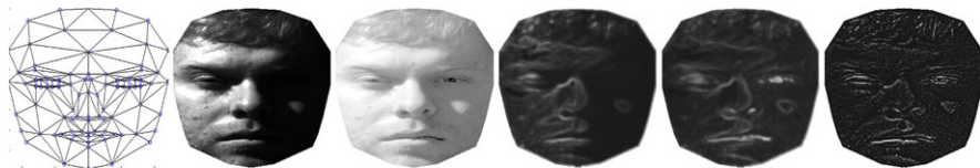
Fig. 6 Normalized face images. From left to right : CANDIDE-3 mesh; normalized face image; gamma corrected image. Ggauss applied to image; Ggauss applied to gamma-corrected image; Illumination normalization applied to image. For better visibility, textures are extracted at 300 \times 300 pixels and adjusted for better contrast
