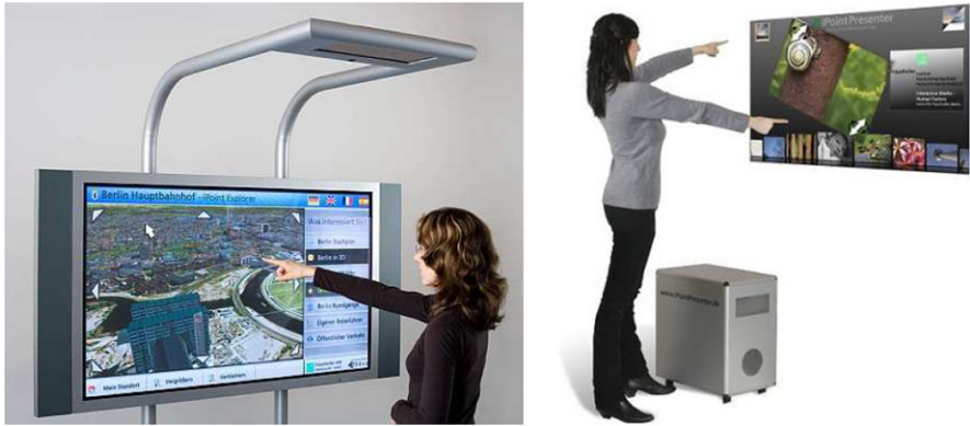
Fig. 12 Gesture interaction systems from Fraunhofer [90]: (Left) iPoint Explorer and (Right) iPoint Presenter
