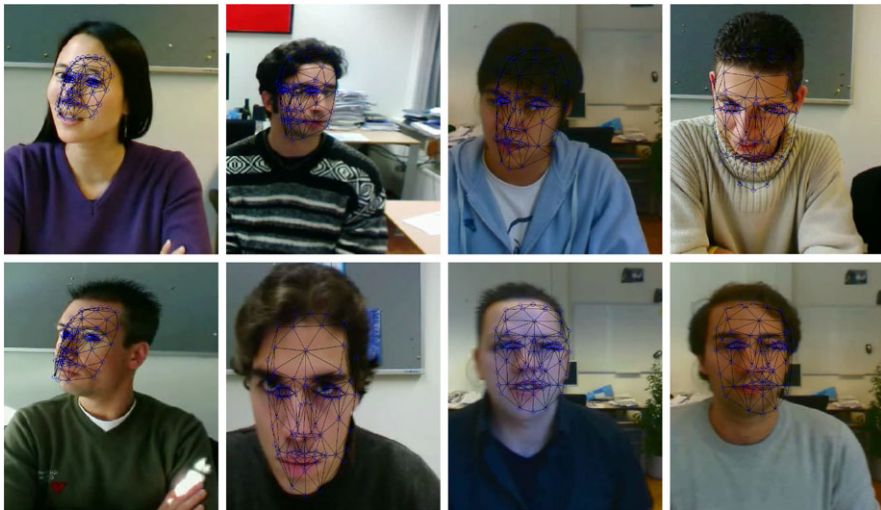
Fig. 18 Examples of bad estimation of mesh pose on the videos used to benchmark the system. All results are obtained with method HS(1)+LK, as shown in Table 2, with texture size of 40 \times 40 pixels, 35 Eigen vectors, and gamma correction followed by Ggauss as texture preprocessing
