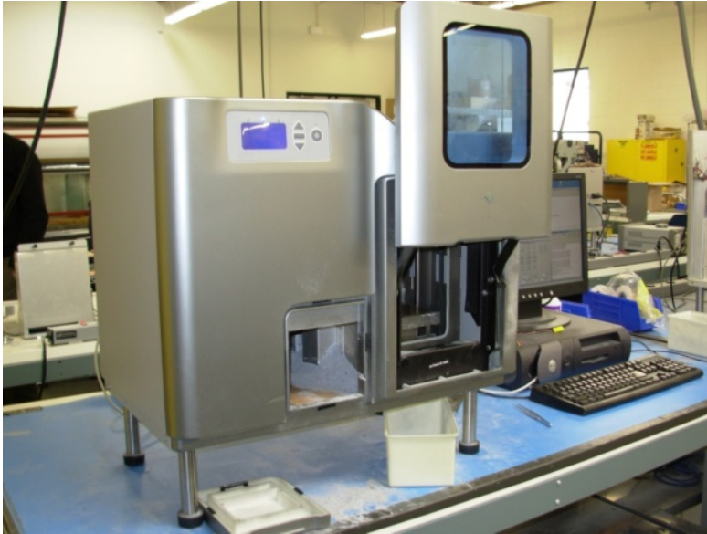
Figure 13.4 Beta test version of desk top factory low cost AM machine (copyright Econolyst Ltd.)
