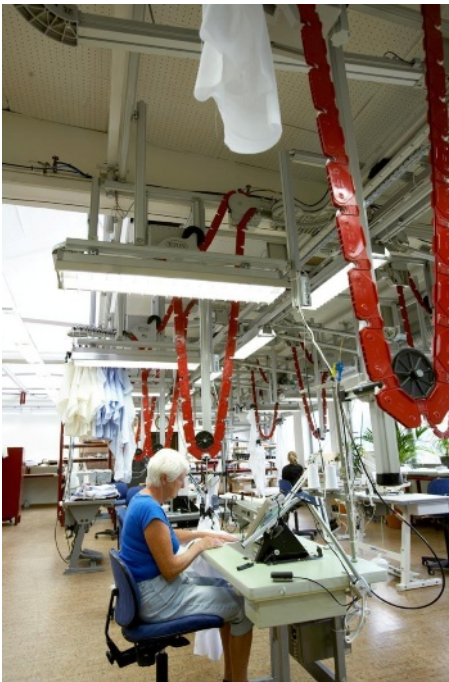
Figure 11.4 The Eton system from Sweden
