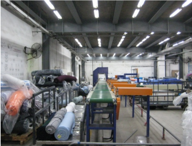
Figure 11.1 Conveyor belt of conveyor MHS
