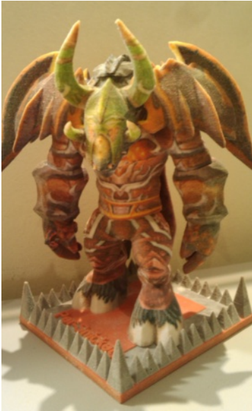
Figure 13.2 World of Warcraft model printed using Z-Corp 3DP (copyright Econolyst Ltd.)
