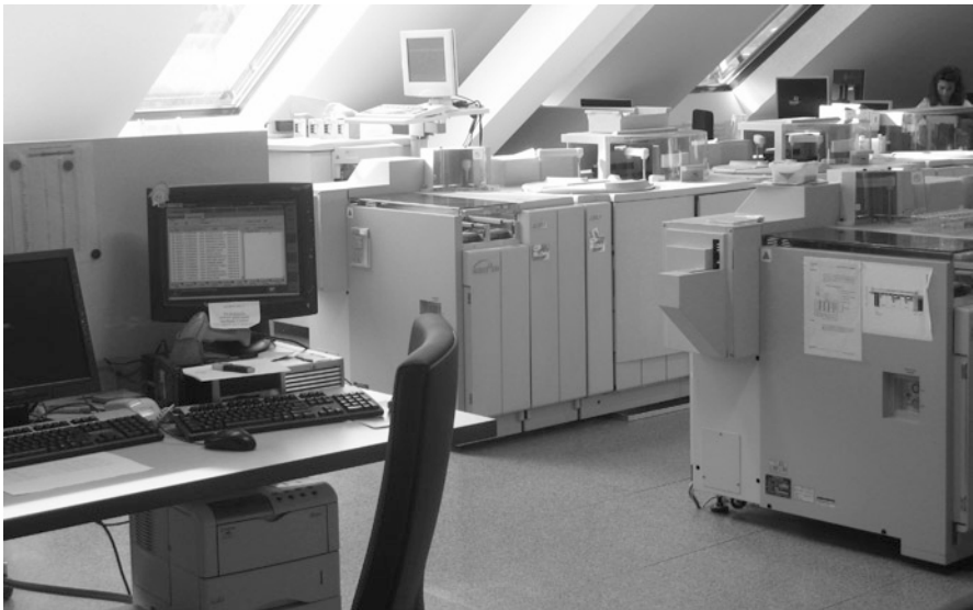
Fig. 6.39 In a laboratory unit. The laboratory information system (LIS; running on the PC in the front) manages the analysis of samples by laboratory devices (in the background)
