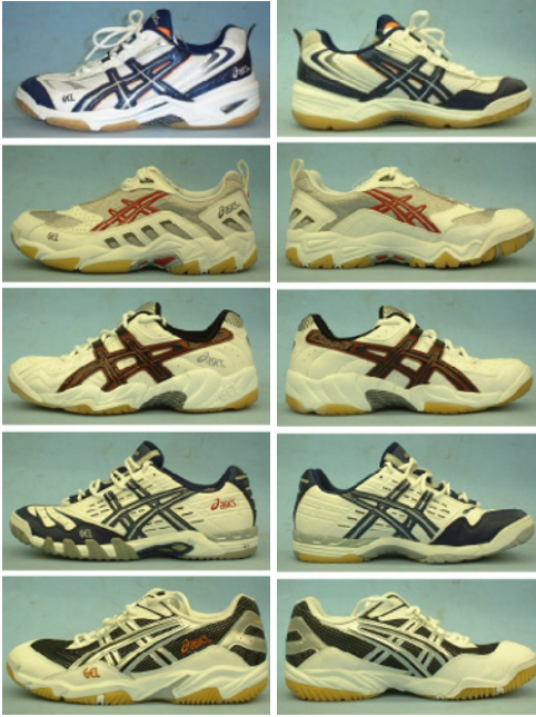
Figure 19.16 Test shoes with different upper material and structures. Shoes are numbered type-1 to 5, beginning at the top
