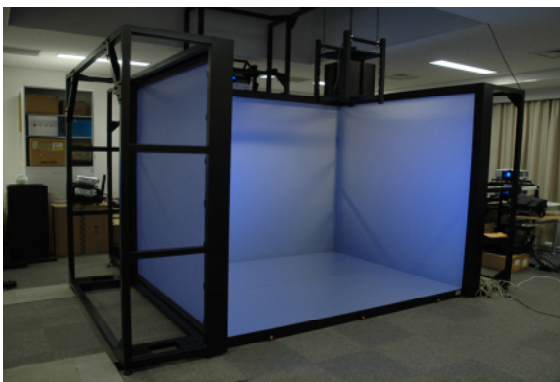
Figure 6.1 Immersive projection display K-Cave
