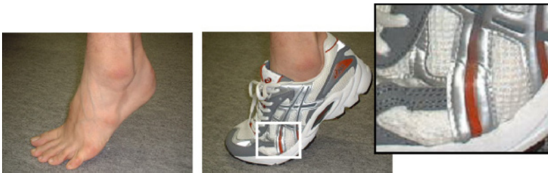
Figure 19.5 Example of deformation of running shoe upper just before toe off. Some wrinkles can be observed in this magnified photo
