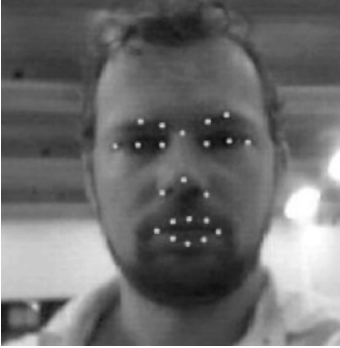
Figure 12.4 FFT-SDK provides 22 feature positions
