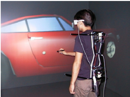
Figure 6.4 Wearable force feedback device HapticGEAR
