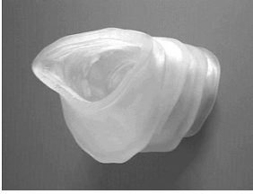
Figure 13.3 Photoformed product made from lip motion data
