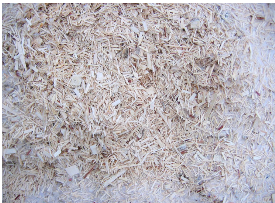
Figure 2.2 Chemically treated wood residues from process industry, which do not contain heavy metals or halogenated organic compounds
