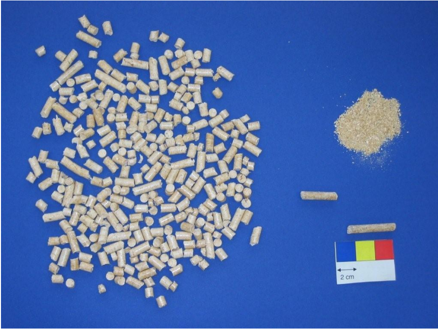
Figure 2.5 Wood pellets classified according to EN 14961-1
