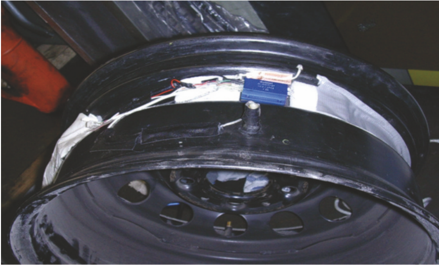
Figure 8.15 Detail of the battery and wireless transmitter installed on the wheel rim
