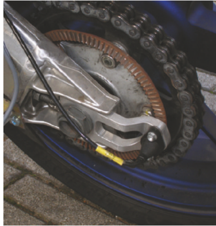
Figure B.1 Example of a wheel encoder installed on a motorbike
