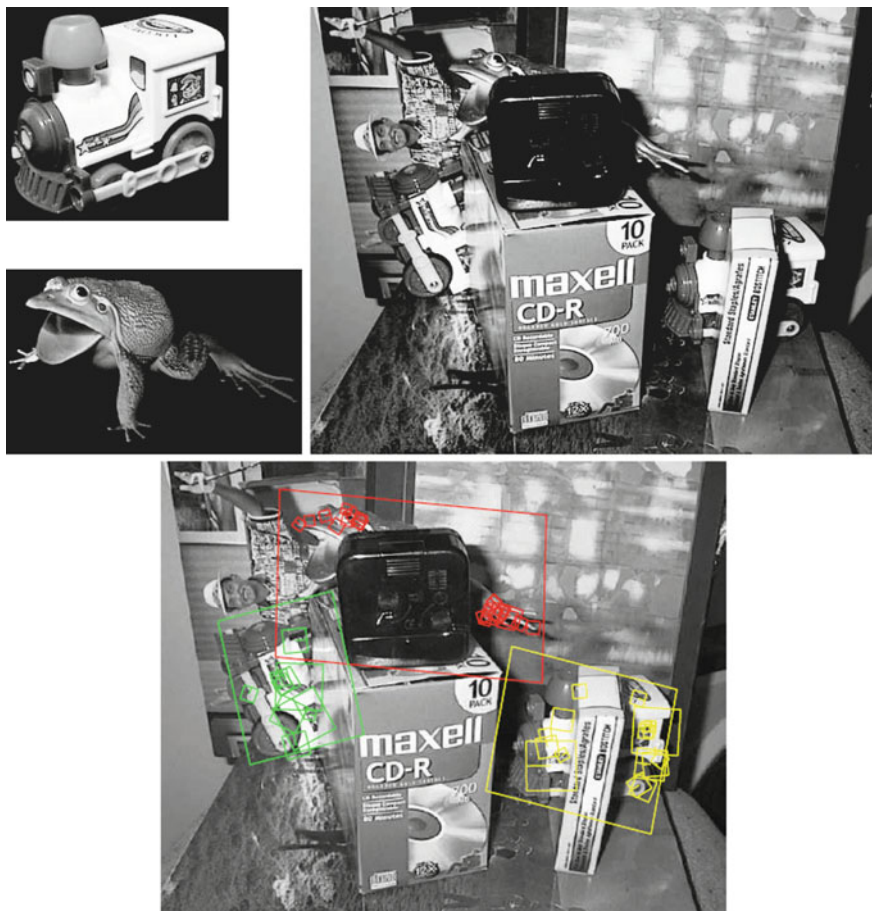
Fig. 7.5 Taken from Lowe [18] 2 illustrating the recognition performance in the presence of heavy occlusion and background clutter
