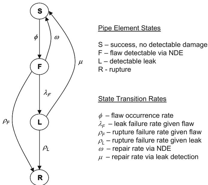
Fig. 13.5 Markov model for piping rupture, taken from [7]
