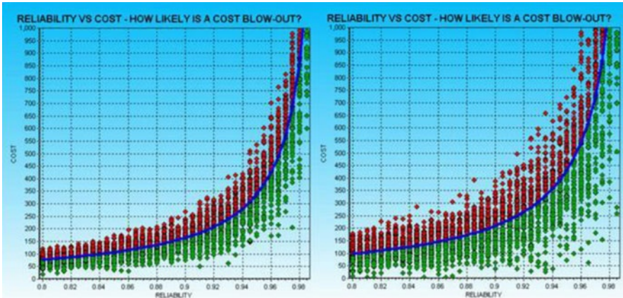
Figure 1 Printed screens from the SACA Concept Demonstrator. Curves for reliability level versus total maintenance costs (dark, continuous line). The scatter around the curve results from the variance of maintenance costs and can be used as an indicator of the risk for cost overruns (above the line) or cost savings (below the line)
