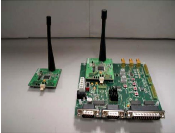
Figure 13 Left CC1010 module, Right CC1010 development board with module attached
