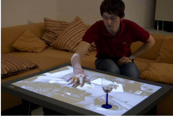
Fig. 11.2 Touches from different users on a DiamondTouch table are distinguished from one another through separate signals broadcast through each user's chair and capacitively coupled through the user into the table's antennas. The table distinguished multiple touches from different users
