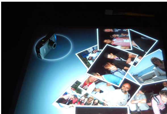
Fig. 11.3 All pictures are sent to the table's surface, once the WiFi-based camera is put on the table
