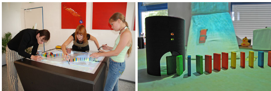
Fig. 11.10 (left) Players have to draw a path on the surface for placing digital domino tiles. (right) Different physical objects have to be used for pushing the real/digital domino pieces. The photo sensor of a tower, for instance, can track the falling physical piece and push the digital ones
