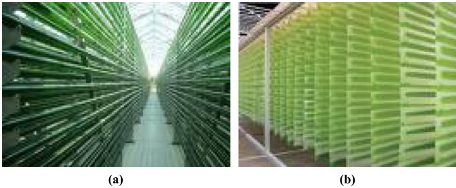
Figure 4.3 (a) Tubular and (b) vertical photobioreactors
