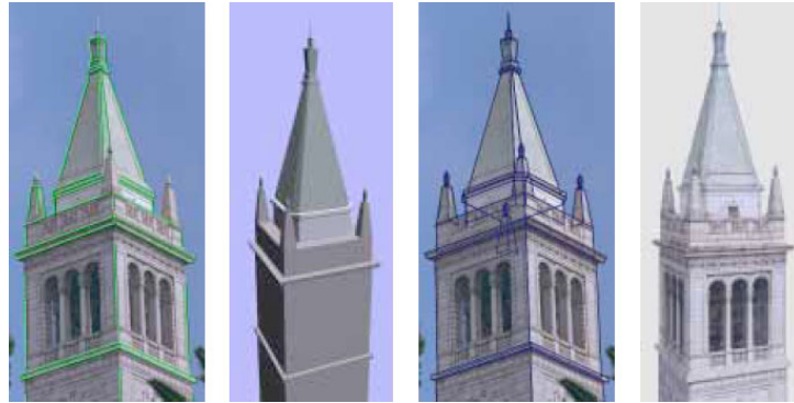
Figure 12.14 Interactive architectural modeling using the Façade system (Debevec, Taylor, and Malik 1996) © 1996 ACM: (a) input image with user-drawn edges shown in green; (b) shaded 3D solid model; (c) geometric primitives overlaid onto the input image; (d) final view-dependent, texture-mapped 3D model.
