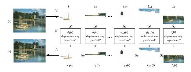
**Figure 13.14** Animating still pictures (Chuang, Goldman, Zheng *et al.* 2005) © 2005 ACM. (a) The input still image is manually segmented into (b) several layers. (c) Each layer is then animated with a different stochastic motion texture (d) The animated layers are then composited to produce (e) the final animation
