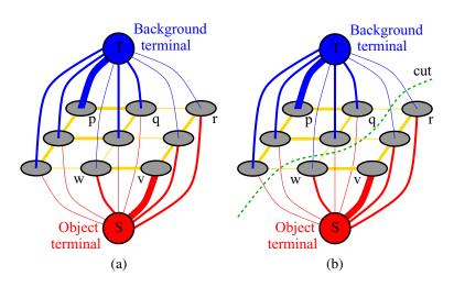
**Figure B.3** Graph cuts for minimizing binary sub-modular MRF energies (Boykov and Jolly 2001) © 2001 IEEE: (a) energy function encoded as a max flow problem; (b) the minimum cut determines the region boundary.
