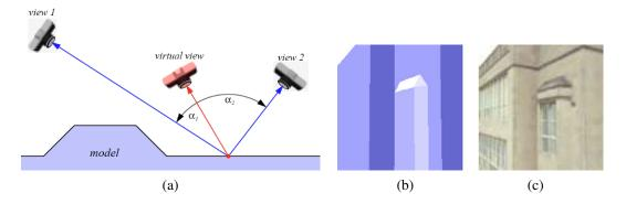
**Figure 13.3** View-dependent texture mapping (Debevec, Taylor, and Malik 1996) © 1996 ACM. (a) The weighting given to each input view depends on the relative angles between the novel (virtual) view and the original views; (b) simplified 3D model geometry; (c) with view-dependent texture mapping, the geometry appears to have more detail (recessed windows).
