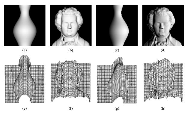
**Figure 12.2** Synthetic shape from shading (Zhang, Tsai, Cryer *et al.* 1999)  $\bigcirc$  1999 IEEE: shaded images, (a–b) with light from in front (0, 0, 1) and (c–d) with light the front right (1, 0, 1); (e–f) corresponding shape from shading reconstructions using the technique of Tsai and Shah (1994).
