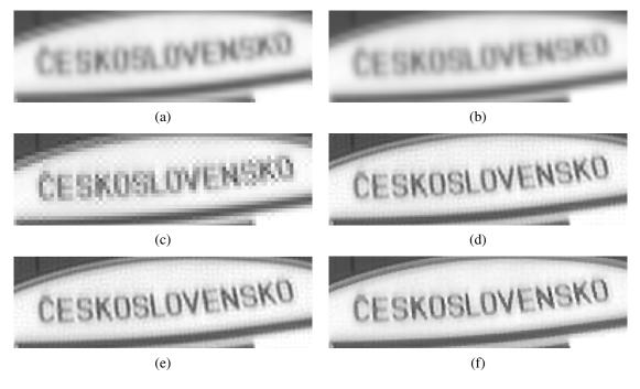
Figure 10.31 Super-resolution results using a variety of image priors (Capel 2001): (a) Low-res ROI (bicubic  $3 \times \text{ zoom}$ ); (b) average image; (c) MLE @  $1.25 \times$  pixel-zoom; (d) simple  $||x||^2$  prior ( $\lambda = 0.004$ ); (e) GMRF ( $\lambda = 0.003$ ); (f) HMRF ( $\lambda = 0.01$ ,  $\alpha = 0.04$ ). 10 images are used as input and a  $3 \times$  super-resolved image is produced in each case, except for the MLE result in (c).
