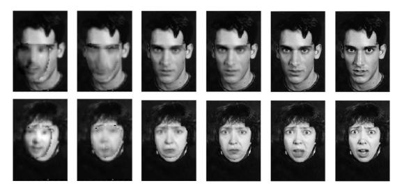
**Figure 14.23** Multiresolution model fitting (search) in active appearance models (Cootes, Edwards, and Taylor 2001) © 2001 IEEE. The columns show the initial model, the results after 3, 8, and 11 iterations, and the final convergence. The rightmost column shows the input image.
