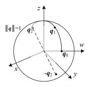
**Figure 2.6** Unit quaternions live on the unit sphere ||q|| = 1. This figure shows a smooth trajectory through the three quaternions  $q_0$ ,  $q_1$ , and  $q_2$ . The *antipodal* point to  $q_2$ , namely  $-q_2$ , represents the same rotation as  $q_2$ .
