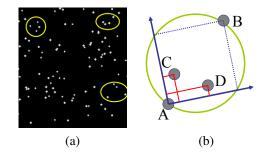
**Figure 14.34** Locating star fields using astrometry, http://astrometry.net/. (a) Input star field and some selected star quads. (b) The 2D coordinates of stars C and D are encoded relative to the unit square defined by A and B.
