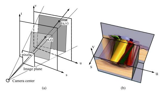
**Figure 13.7** The Lumigraph (Gortler, Grzeszczuk, Szeliski *et al.* 1996)  $\bigcirc$  1996 ACM: (a) a ray is represented by its 4D two-plane parameters (s, t) and (u, v); (b) a slice through the 3D light field subset (u, v, s).
