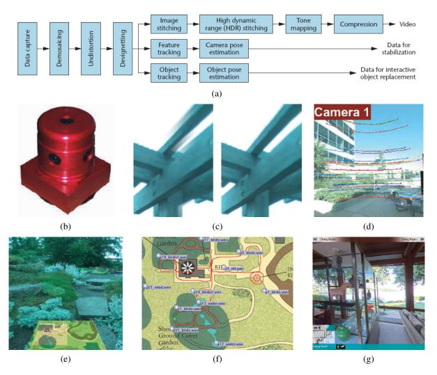
**Figure 13.16** Video-based walkthroughs (Uyttendaele, Criminisi, Kang *et al.* 2004)  $\bigcirc$  2004 IEEE: (a) system diagram of video pre-processing; (b) the Point Grey Ladybug camera; (c) ghost removal using multi-perspective plane sweep; (d) point tracking, used both for calibration and stabilization; (e) interactive garden walkthrough with map below; (f) overhead map authoring and sound placement; (g) interactive home walkthrough with navigation bar (top) and icons of interest (bottom).
