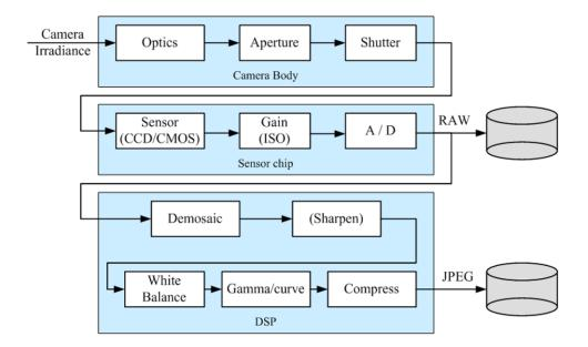
Figure 2.23 Image sensing pipeline, showing the various sources of noise as well as typical digital post-processing steps.
