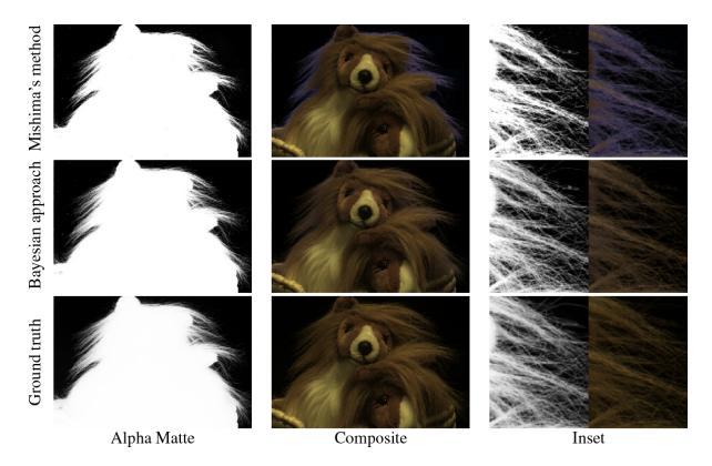
**Figure 10.40** Blue-screen matting results (Chuang, Curless, Salesin *et al.* 2001) © 2001 IEEE. Mishima's method produces visible blue spill (color fringing in the hair), while Chuang's Bayesian matting approach produces accurate results.
