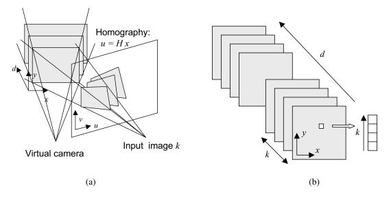
**Figure 11.6** Sweeping a set of planes through a scene (Szeliski and Golland 1999)  $\bigcirc$  1999 Springer: (a) The set of planes seen from a virtual camera induces a set of homographies in any other source (input) camera image. (b) The warped images from all the other cameras can be stacked into a generalized disparity space volume  $\tilde{I}(x, y, d, k)$  indexed by pixel location (x, y), disparity d, and camera k.
