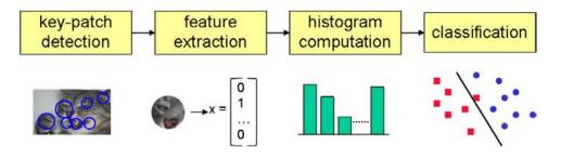
**Figure 14.36** A typical processing pipeline for a bag-of-words category recognition system (Csurka, Dance, Perronnin *et al.* 2006) © 2007 Springer. Features are first extracted at keypoints and then quantized to get a distribution (histogram) over the learned *visual words* (feature cluster centers). The feature distribution histogram is used to learn a decision surface using a classification algorithm, such as a support vector machine.
