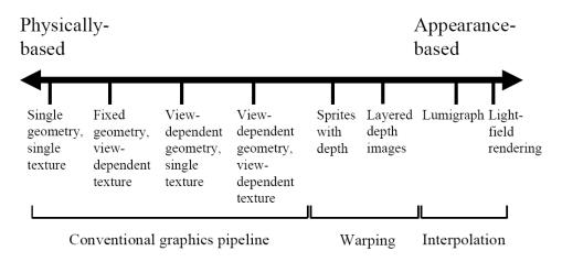
**Figure 13.11** The geometry-image continuum in image-based rendering (Kang, Szeliski, and Anandan 2000) © 2000 IEEE. Representations at the left of the spectrum use more detailed geometry and simpler image representations, while representations and algorithms on the right use more images and less geometry.
