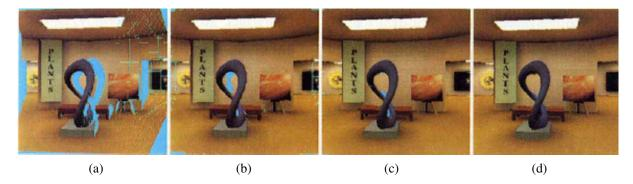
**Figure 13.2** View interpolation (Chen and Williams 1993) © 1993 ACM: (a) holes from one source image (shown in blue); (b) holes after combining two widely spaced images; (c) holes after combining two closely spaced images; (d) after interpolation (hole filling).
