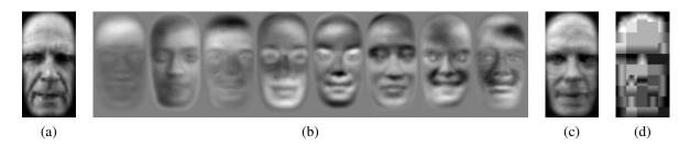
**Figure 14.13** Face modeling and compression using eigenfaces (Moghaddam and Pentland 1997) © 1997 IEEE: (a) input image; (b) the first eight eigenfaces; (c) image reconstructed by projecting onto this basis and compressing the image to 85 bytes; (d) image reconstructed using JPEG (530 bytes).
