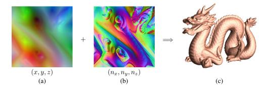
**Figure 12.12** Geometry images (Gu, Gortler, and Hoppe 2002) C 2002 ACM: (a) the 257 × 257 geometry image defines a mesh over the surface; (b) the 512 × 512 normal map defines vertex normals; (c) final lit 3D model.
