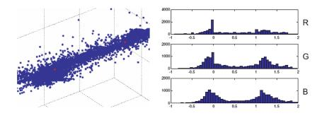
**Figure 10.36** Two-color model computed from a collection of local  $5 \times 5$  neighborhoods (Bennett, Uyttendaele, Zitnick *et al.* 2006) © 2006 Springer. After two-means clustering and reprojection along the line joining the two dominant colors (red dots), the majority of the pixels fall near the fitted line. The distribution along the line, projected along the RGB axes, is peaked at 0 and 1, the two dominant colors.
