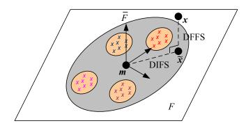
**Figure 14.14** Projection onto the linear subspace spanned by the eigenface images (Moghaddam and Pentland 1997) © 1997 IEEE. The distance from face space (DFFS) is the orthogonal distance to the plane, while the distance in face space (DIFS) is the distance along the plane from the mean image. Both distances can be turned into Mahalanobis distances and given probabilistic interpretations.
