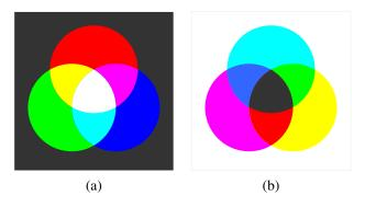
**Figure 2.27** Primary and secondary colors: (a) additive colors red, green, and blue can be mixed to produce cyan, magenta, yellow, and white; (b) subtractive colors cyan, magenta, and yellow can be mixed to produce red, green, blue, and black.
