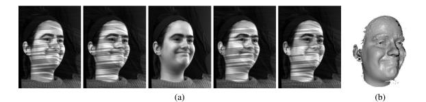
**Figure 12.7** Real-time dense 3D face capture using spacetime stereo (Zhang, Snavely, Curless *et al.* 2004) © 2004 ACM: (a) set of five consecutive video frames from one of two stereo cameras (every fifth frame is free of stripe patterns, in order to extract texture); (b) resulting high-quality 3D surface model (depth map visualized as a shaded rendering).
