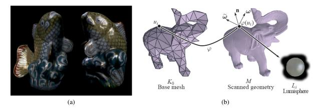
**Figure 13.9** Surface light fields (Wood, Azuma, Aldinger *et al.* 2000) © 2000 ACM: (a) example of a highly specular object with strong inter-reflections; (b) the surface light field stores the light emanating from each surface point in all visible directions as a "Lumisphere".
