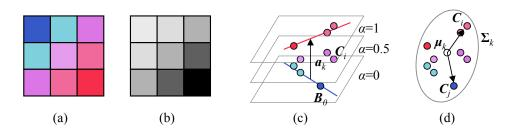
Figure 10.43 Color line matting (Levin, Lischinski, and Weiss 2008): (a) local  $3 \times 3$  patch of colors; (b) potential assignment of  $\alpha$  values; (c) foreground and background color lines, the vector  $a_k$  joining their closest points of intersection, and the family of parallel planes of constant  $\alpha$  values,  $\alpha_i = a_k \cdot (C_i - B_0)$ ; (d) a scatter plot of sample colors and the deviations from the mean  $\mu_k$  for two sample colors  $C_i$  and  $C_j$ .
