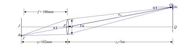
**Figure 2.22** The amount of light hitting a pixel of surface area  $\delta i$  depends on the square of the ratio of the aperture diameter d to the focal length f, as well as the fourth power of the off-axis angle  $\alpha$  cosine,  $\cos^4 \alpha$ .
