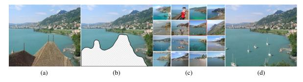
**Figure 14.46** Scene completion using millions of photographs (Hays and Efros 2007) © 2007 ACM: (a) original image; (b) after unwanted foreground removal; (c) plausible scene matches, with the one the user selected highlighted in red; (d) output image after replacement and blending.
