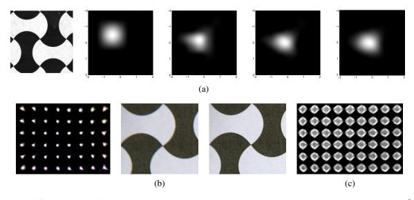
**Figure 10.8** Point spread function estimation using a calibration target (Joshi, Szeliski, and Kriegman 2008) © 2008 IEEE. (a) Sub-pixel PSFs at successively higher resolutions (note the interaction between the square sensing area and the circular lens blur). (b) The radial distortion and chromatic aberration can also be estimated and removed. (c) PSF for a mis-focused (blurred) lens showing some diffraction and vignetting effects in the corners.
