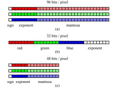
**Figure 10.19** HDR image encoding formats: (a) Portable PixMap (.ppm); (b) Radiance (.pic, .hdr); (c) OpenEXR (.exr).
