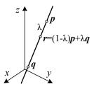
Figure 2.3 3D line equation,  $r = (1 - \lambda)p + \lambda q$ .
