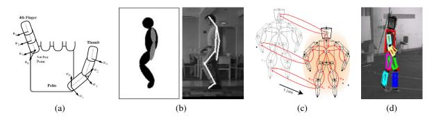
**Figure 12.20** Tracking 3D human motion: (a) kinematic chain model for a human hand (Rehg, Morris, and Kanade 2003) © 2003, reprinted by permission of SAGE; (b) tracking a kinematic chain blob model in a video sequence (Bregler, Malik, and Pullen 2004) © 2004 Springer; (c–d) probabilistic loose-limbed collection of body parts (Sigal, Bhatia, Roth *et al.* 2004)
