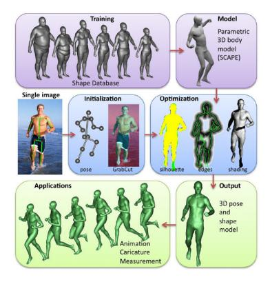
**Figure 12.21** Estimating human shape and pose from a single image using a parametric 3D model (Guan, Weiss, Bălan *et al.* 2009) (c) 2009 IEEE.
