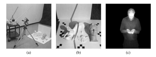
**Figure 12.6** Shape scanning using cast shadows (Bouguet and Perona 1999) (c) 1999 Springer: (a) camera setup with a point light source (a desk lamp without its reflector), a hand-held stick casting a shadow, and (b) the objects being scanned in front of two planar backgrounds. (c) Real-time depth map using a pulsed illumination system (Iddan and Yahay 2001) (c) 2001 SPIE.
