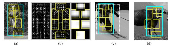
**Figure 14.9** Part-based object detection (Felzenszwalb, McAllester, and Ramanan 2008) © 2008 IEEE: (a) An input photograph and its associated person (blue) and part (yellow) detection results. (b) The detection model is defined by a coarse template, several higher resolution part templates, and a spatial model for the location of each part. (c) True positive detection of a skier and (d) false positive detection of a cow (labeled as a person).
