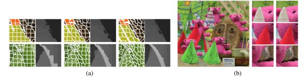
**Figure 11.13** Stereo matching with adaptive over-segmentation and matting (Taguchi, Wilburn, and Zitnick 2008) © 2008 IEEE: (a) segment boundaries are refined during the optimization, leading to more accurate results (e.g., the thin green leaf in the bottom row); (b) alpha mattes are extracted at segment boundaries, which leads to visually better compositing results (middle column).
