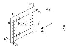
**Figure 2.9** Simplified camera intrinsics showing the focal length f and the optical center  $(c_x, c_y)$ . The image width and height are W and H.
