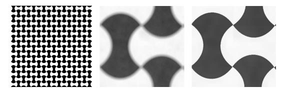
**Figure 10.7** Calibration pattern with edges equally distributed at all orientations that can be used for PSF and radial distortion estimation (Joshi, Szeliski, and Kriegman 2008) © 2008 IEEE. A portion of an actual sensed image is shown in the middle and a close-up of the ideal pattern is on the right.
