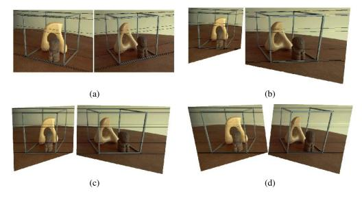
**Figure 11.4** The multi-stage stereo rectification algorithm of Loop and Zhang (1999) © 1999 IEEE. (a) Original image pair overlaid with several epipolar lines; (b) images transformed so that epipolar lines are parallel; (c) images rectified so that epipolar lines are horizontal and in vertial correspondence; (d) final rectification that minimizes horizontal distortions.
