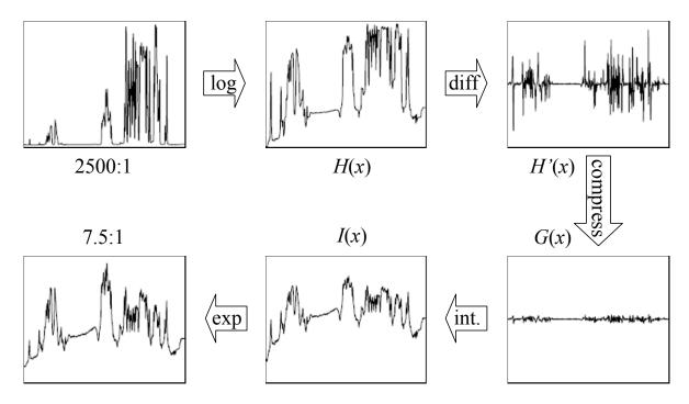
**Figure 10.25** Gradient domain tone mapping (Fattal, Lischinski, and Werman 2002) © 2002 ACM. The original image with a dynamic range of 2415:1 is first converted into the log domain, H(x), and its gradients are computed, H'(x). These are attenuated (compressed) based on local contrast, G(x), and integrated to produce the new logarithmic exposure image I(x), which is exponentiated to produce the final intensity image, whose dynamic range is 7.5:1.
