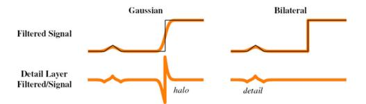
**Figure 10.23** Gaussian vs. bilateral filtering (Petschnigg, Agrawala, Hoppe *et al.* 2004) © 2004 ACM: A Gaussian low-pass filter blurs across all edges and therefore creates strong peaks and valleys in the detail image that cause halos. The bilateral filter does not smooth across strong edges and thereby reduces halos while still capturing detail.
