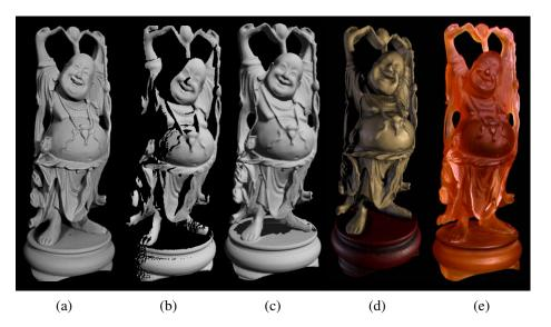
**Figure 12.9** Reconstruction and hardcopy of the "Happy Buddha" statuette (Curless and Levoy 1996) © 1996 ACM: (a) photograph of the original statue after spray painting with matte gray; (b) partial range scan; (c) merged range scans; (d) colored rendering of the reconstructed model; (e) hardcopy of the model constructed using stereolithography.
