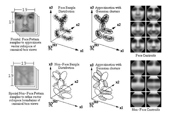
**Figure 14.4** Learning a mixture of Gaussians model for face detection (Sung and Poggio 1998)  $\bigcirc$  1998 IEEE. The face and non-face images (19<sup>2</sup>-long vectors) are first clustered into six separate clusters (each) using k-means and then analyzed using PCA. The cluster centers are shown in the right-hand columns.
