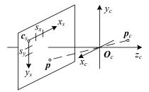
**Figure 2.8** Projection of a 3D camera-centered point  $p_c$  onto the sensor planes at location p.  $O_c$  is the camera center (nodal point),  $c_s$  is the 3D origin of the sensor plane coordinate system, and  $s_x$  and  $s_y$  are the pixel spacings.
