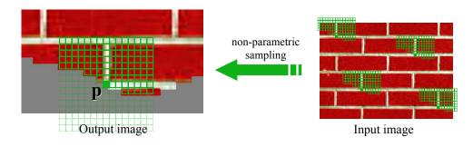
Figure 10.50 Texture synthesis using non-parametric sampling (Efros and Leung 1999). The value of the newest pixel p is randomly chosen from similar local (partial) patches in the source texture (input image). (Figure courtesy of Alyosha Efros.)
