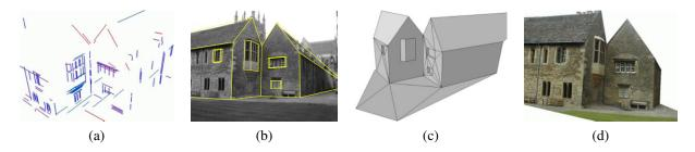
**Figure 12.16** Automated architectural reconstruction using 3D lines and planes (Werner and Zisserman 2002) © 2002 Springer: (a) reconstructed 3D lines, color coded by their vanishing directions; (b) wire-frame model superimposed onto an input image; (c) triangulated piecewise-planar model with windows; (d) final texture-mapped model.
