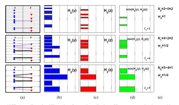
**Figure 14.38** A one-dimensional illustration of comparing collections of feature vectors using the pyramid match kernel (Grauman and Darrell 2007b): (a) distribution of feature vectors (point sets) into the pyramidal bins; (b–c) histogram of point counts in bins  $B_{il}$  and  $B'_{il}$  for the two images; (d) histogram intersections (minimum values); (e) per-level similarity scores, which are weighted and summed to form the final distance/similarity metric.
