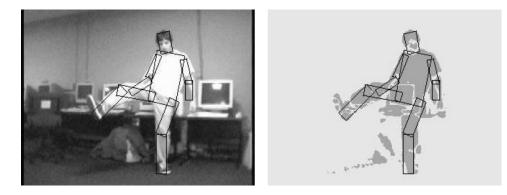
**Figure 14.40** Using pictorial structures to locate and track a person (Felzenszwalb and Huttenlocher 2005) © 2005 Springer. The structure consists of articulated rectangular body parts (torso, head, and limbs) connected in a tree topology that encodes relative part positions and orientations. To fit a pictorial structure model, a binary silhouette image is first computed using background subtraction.
