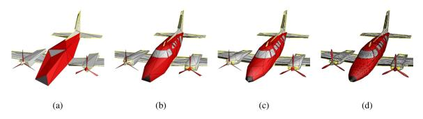
**Figure 12.11** Progressive mesh representation of an airplane model (Hoppe 1996)  $\bigcirc$  1996 ACM: (a) base mesh  $M^0$  (150 faces); (b) mesh  $M^{175}$  (500 faces); (c) mesh  $M^{425}$  (1000 faces); (d) original mesh  $M = M^n$  (13,546 faces).
