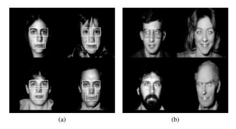
**Figure 14.18** Modular eigenspace for face recognition (Moghaddam and Pentland 1997) © 1997 IEEE. (a) By detecting separate features in the faces (eyes, nose, mouth), separate eigenspaces can be estimated for each one. (b) The relative positions of each feature can be detected at recognition time, thus allowing for more flexibility in viewpoint and expression.
