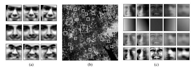
**Figure 14.3** Pre-processing stages for face detector training (Rowley, Baluja, and Kanade 1998a) © 1998 IEEE: (a) artificially mirroring, rotating, scaling, and translating training images for greater variability; (b) using images without faces (looking up at a tree) to generate non-face examples; (c) pre-processing the patches by subtracting a best fit linear function (constant gradient) and histogram equalizing.
