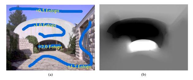
**Figure 10.28** Interactive local tone mapping (Lischinski, Farbman, Uyttendaele *et al.* 2006b) © 2006 ACM: (a) user-drawn strokes with associated exposure values g(x, y) (b) corresponding piecewise-smooth exposure adjustment map f(x, y).
