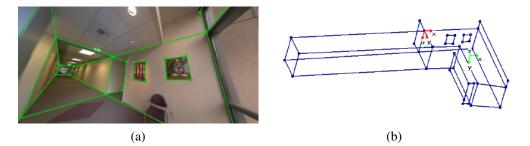
**Figure 12.15** Interactive 3D modeling from panoramas (Shum, Han, and Szeliski 1998) © 1998 IEEE: (a) wide-angle view of a panorama with user-drawn vertical and horizontal (axis-aligned) lines; (b) single-view reconstruction of the corridors.
