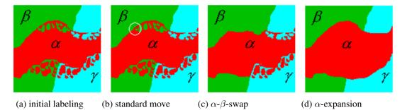
**Figure B.4** Multi-level graph optimization from (Boykov, Veksler, and Zabih 2001)  $\bigcirc$  2001 IEEE: (a) initial problem configuration; (b) the standard move changes only one pixel; (c) the  $\alpha$ - $\beta$ -swap optimally exchanges all  $\alpha$ - and  $\beta$ -labeled pixels; (d) the  $\alpha$ -expansion move optimally selects among current pixel values and the  $\alpha$  label.
