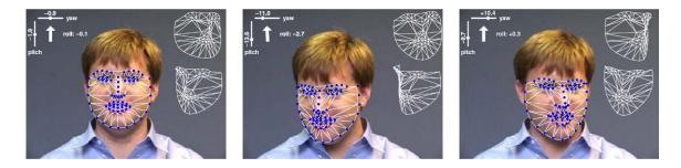
**Figure 14.24** Head tracking with 3D AAMs (Matthews, Xiao, and Baker 2007) © 2007 Springer. Each image shows a video frame along with the estimate yaw, pitch, and roll parameters and the fitted 3D deformable mesh.
