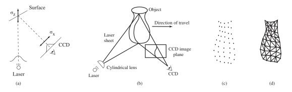
**Figure 12.5** Range data scanning (Curless and Levoy 1996) © 1996 ACM: (a) a laser dot on a surface is imaged by a CCD sensor; (b) a laser stripe (sheet) is imaged by the sensor (the deformation of the stripe encodes the distance to the object); (c) the resulting set of 3D points are turned into (d) a triangulated mesh.
