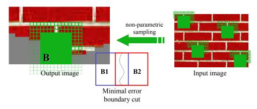
**Figure 10.51** Texture synthesis by image quilting (Efros and Freeman 2001). Instead of generating a single pixel at a time, larger blocks are copied from the source texture. The transitions in the overlap regions between the selected blocks are then optimized using dynamic programming. (Figure courtesy of Alyosha Efros.)
