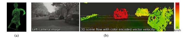
**Figure 11.18** Three-dimensional scene flow: (a) computed from a multi-camera dome surrounding the dancer shown in Figure 11.2h–j (Vedula, Baker, Rander *et al.* 2005) © 2005 IEEE; (b) computed from stereo cameras mounted on a moving vehicle (Wedel, Rabe, Vaudrey *et al.* 2008) © 2008 Springer.
