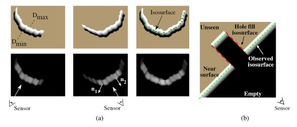
**Figure 12.8** Range data merging (Curless and Levoy 1996)  $\bigcirc$  1996 ACM: (a) two signed distance functions (top left) are merged with their (weights) bottom left to produce a combined set of functions (right column) from which an isosurface can be extracted (green dashed line); (b) the signed distance functions are combined with empty and unseen space labels to fill holes in the isosurface.
