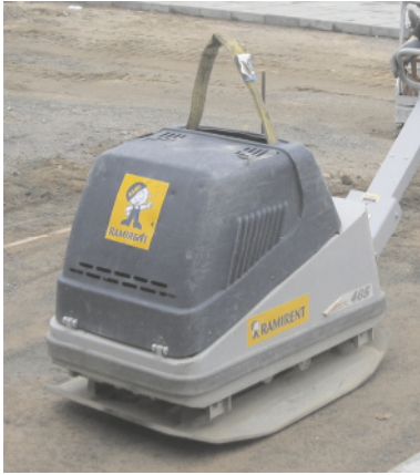
Fig. 3.8 The FB-455 soil compactor in use with the transport textile strap erected (modified from Sundin et al. (2009)).
