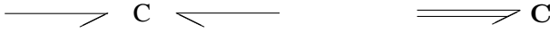
Fig. 8.6 C energy store with two power ports and its representation in a multibond graph
