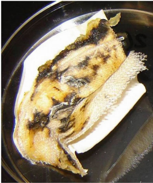
Fig. 8.4 An example of an explanted composite mesh (heavyweight polypropylene/PTFE) after cleaning
