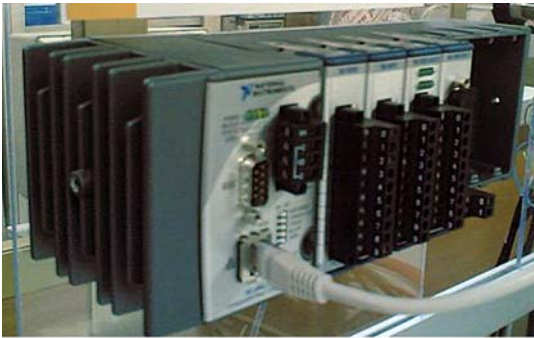
Fig. 1.6a,b Acquisition systems developed by NI [16]. a CompactRIO™. b NI USB DAQ
