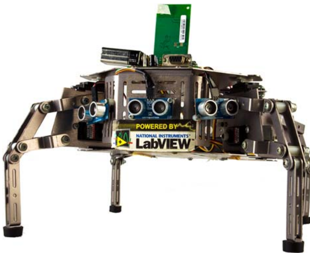
Fig. 5.17 Robot Zil I was controlled by a Fuzzy Logic Controller adjusted using Genetic AlgorithmsC
