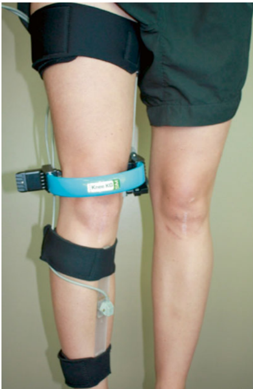
Fig. 39.2 The tibial and femoral components of the KneeKG™ attachment system
