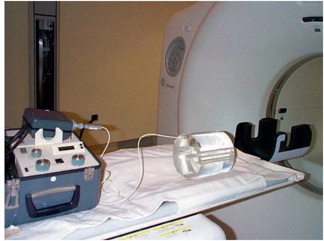
Figure 3.1. A 100-mm length cylindrical acrylic phantom used for measuring the CTDI_{100} .
