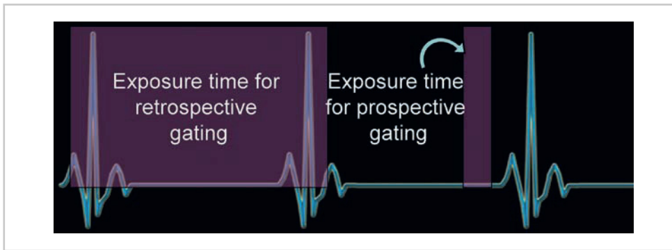
Figure 12.4. Schematic demonstration of the radiation exposure time differences between retrospective gating (single heart beat) and prospective triggering used in wide coverage MDCT scanners.
