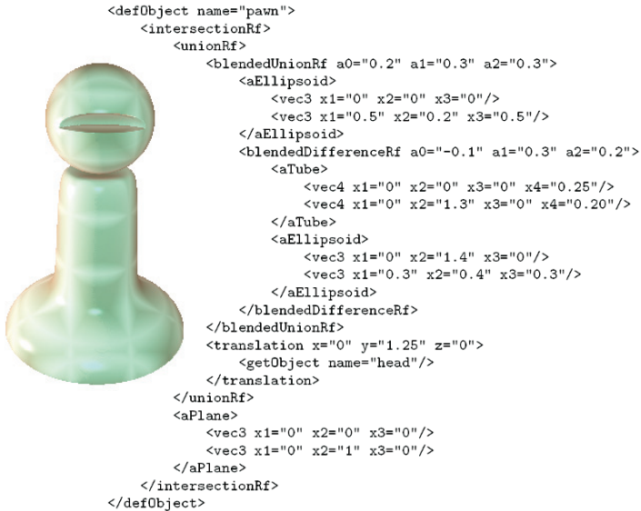
Fig. 2. A demonstration of the XISL language (script) that defines the implicit “pawn” object and the rendered image of the script.
