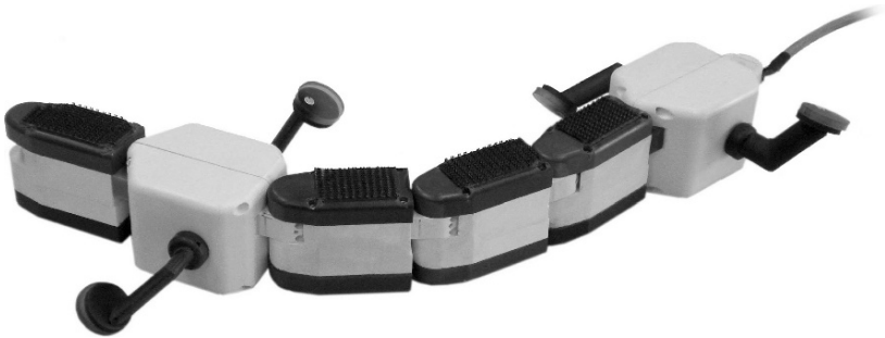
Fig. 3.5 The prototype of salamander robot built with the first generation elements
