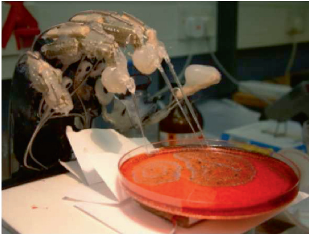
Fig. 11.16 Robotic hand interacts with Belousov–Zhabotinsky medium. From [4]
