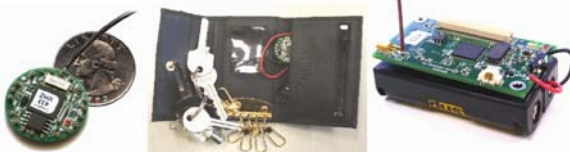
Fig. 15.6 From left to right: mica2dot mote, key-fold with mica2dot, and mica2 mote
