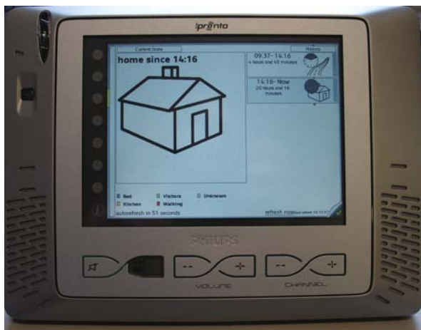
Fig. 15.8 Daily Activities Diarist displayed on a Philips iPronto device, showing the current state ( left ) and the history ( right )
