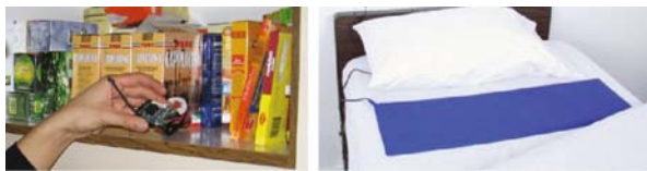
Fig. 15.7 Placing a wireless mote with a photo sensor in a cupboard ( left ), an illustration of a pressure-pad used for bed-activity detection ( right )
