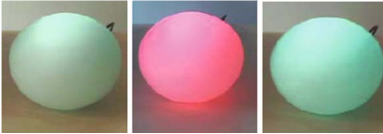
Fig. 19.2 Orb ( top ) and Ticker ( bottom ) sequence shown illustrates (a) a display with no unread e-mails, (b) the display showing the arrival of a new e-mail from Ashley, titled “Let’s meet for lunch.”, and (c) the display showing one unread e-mail
