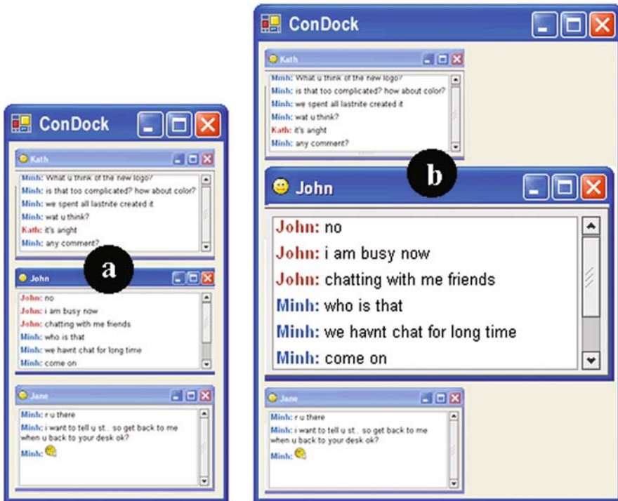
Fig. 13.3 Conversion Dock (ConDock): (a) normal view and (b) magnified view
