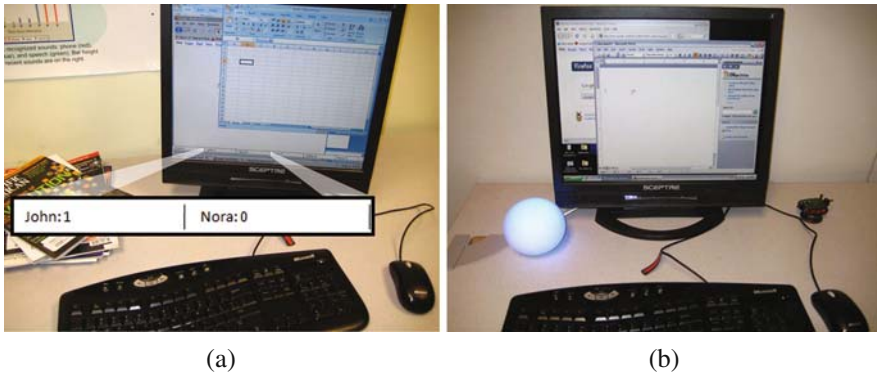
Fig. 19.1 The Ticker and Orb displays. (a) The Ticker, shown in a magnified callout, is located just above the windows taskbar. (b) The Orb is the pink globe to the right of the monitor
