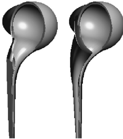
Fig. 10.11. Creating the aperture. Left: the opening which is carved out by Equation (10.20). Right: the final shape of the opening after adding in B_{\text{insidewall}} as in Equation (10.21).
